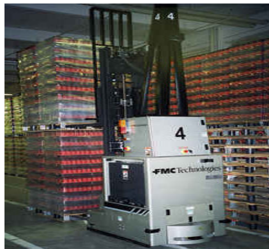
Figure 3.1. An AGV executing a transport task (photo by FMC Technologies).
