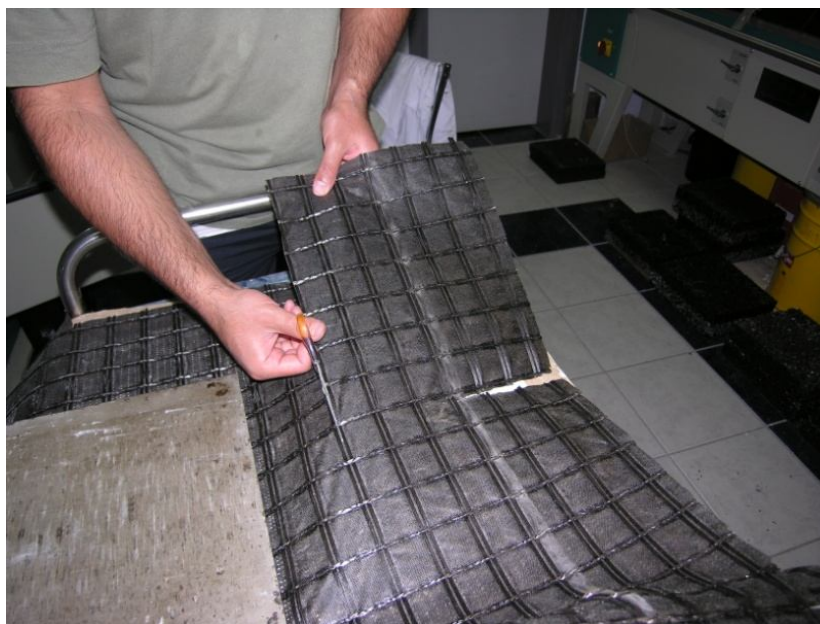
Figure 6.6. Preparation of geosynthetics for test: Cutting of material
