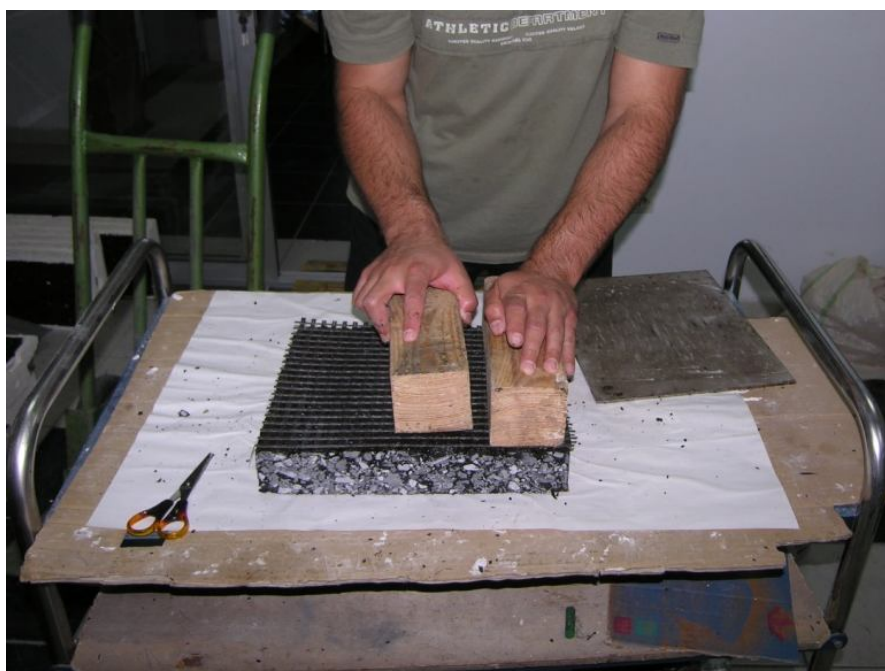
Figure 6.7. Preparation of geosynthetic for test: Installing of geosynthetics
