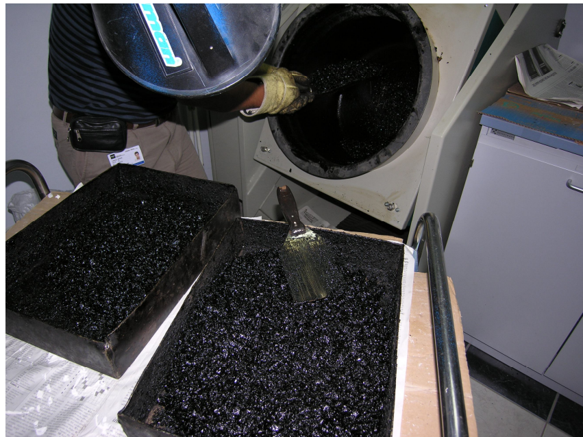
Figure 6.8. Mixing stage of aggregate and bitumen
