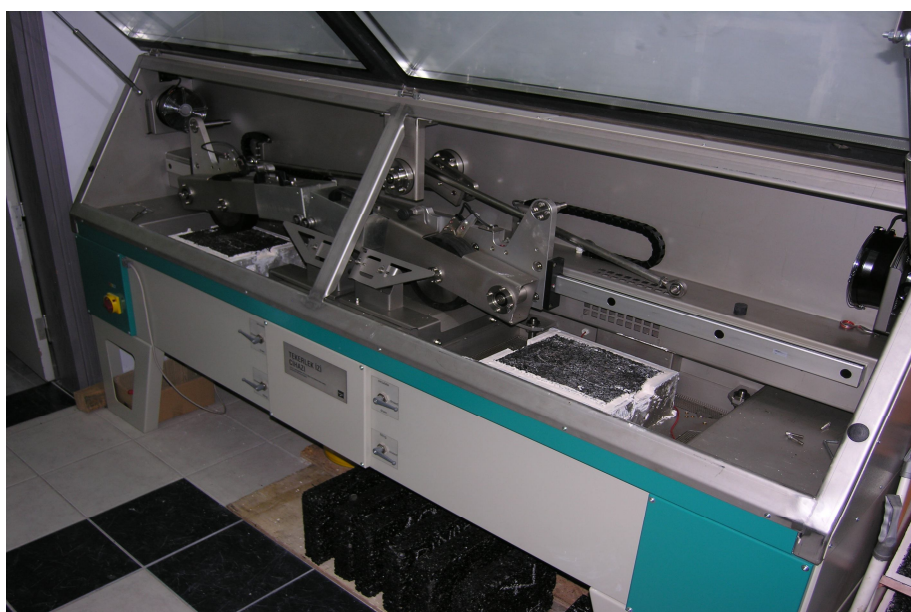
Figure 6.10. Rutting Test of Two Same Plastered Specimens in HWTD
