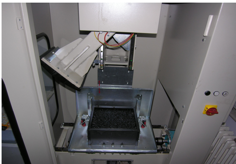
Figure 6.9. Compaction of slabs in segmental compactor.
