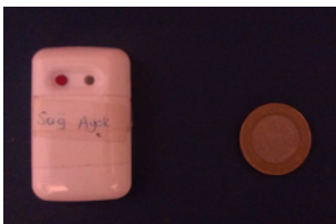
Figure 2.1. ExL IMUs utilized in this study.
