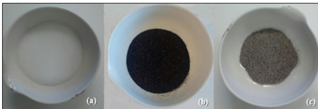
Figure 3.2. The formation of particulate Mn/Na 2 WO 4 /SiO 2 catalyst; (a) 60-100 mesh size silica gel, (b) particulate Mn/Na 2 WO 4 /SiO 2 catalyst after drying at 130 °C, (c) particulate Mn/Na 2 WO 4 /SiO 2 catalyst after calcination at 800 °C.
