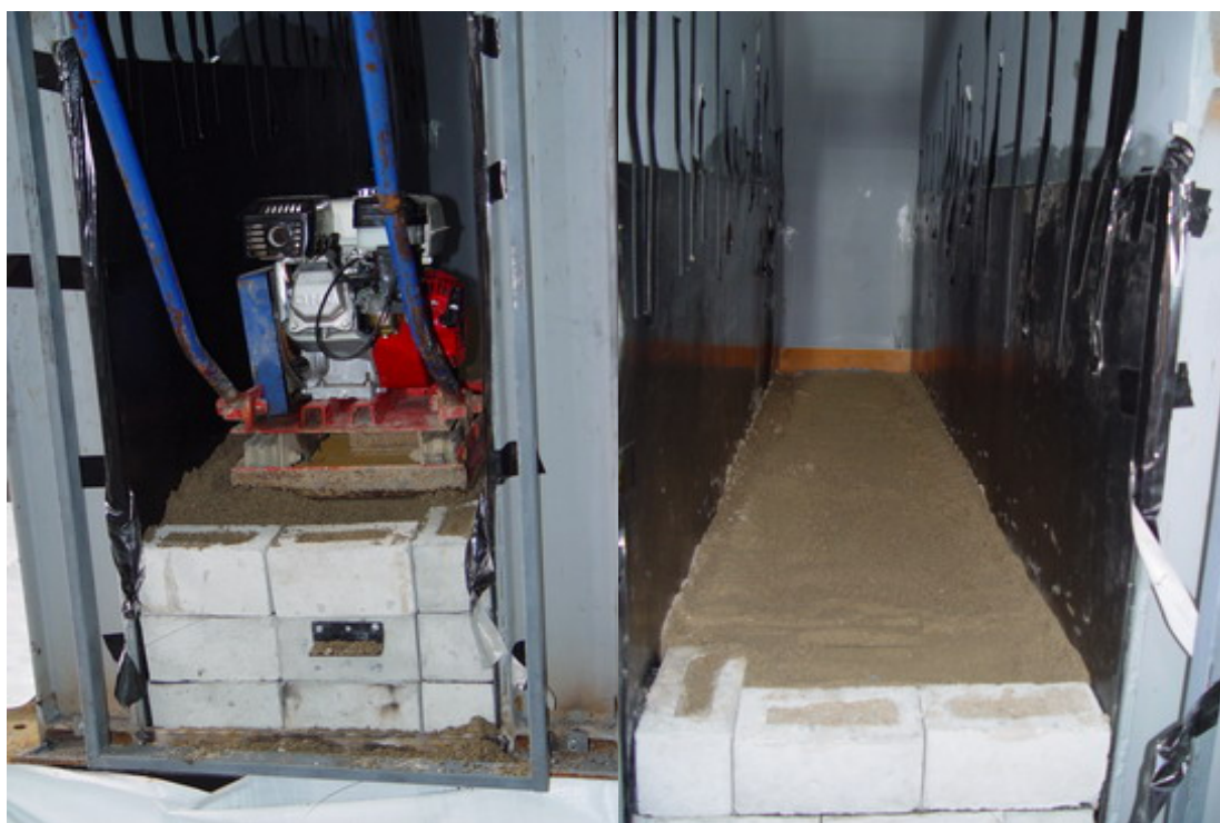
Figure 7.20. The compaction process and the resultant compacted layer.
