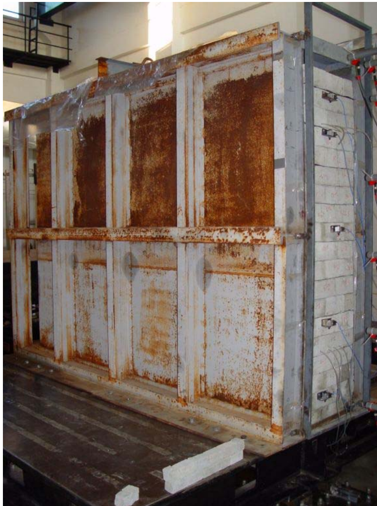
Figure 7.4. Steel container on the shaking table
