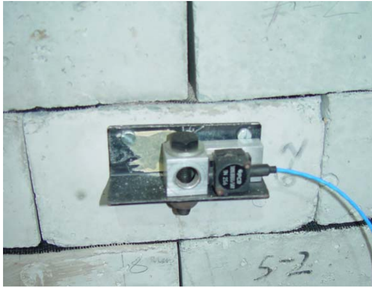
Figure 7.28. The accelerometer mounted onto the surface as shown.
