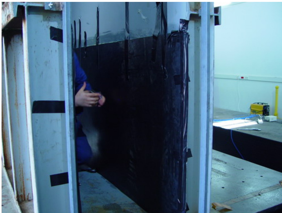
Figure 7.19. Rubber sheets were placed after the lubrication of the side surfaces.
