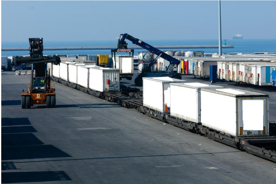
Figure 13. Trailers loading to dedicated train in the seaport by a crane
