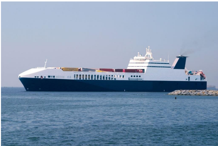
Figure 12. Roro vessel transports trailers
