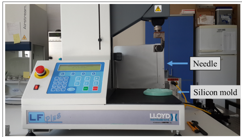
Figure 2.10 Stiffness testing mechanism (LLOYD instruments, LF Plus digital testing machine).
