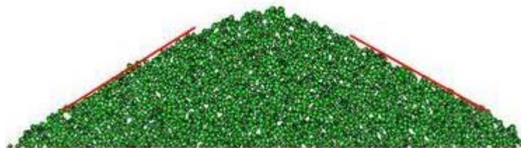
Figure 7.8. Obtaining angle of repose value from numerical experiment
