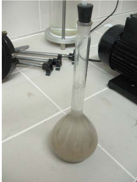
Figure 3.8. Specific gravity experiment setup
