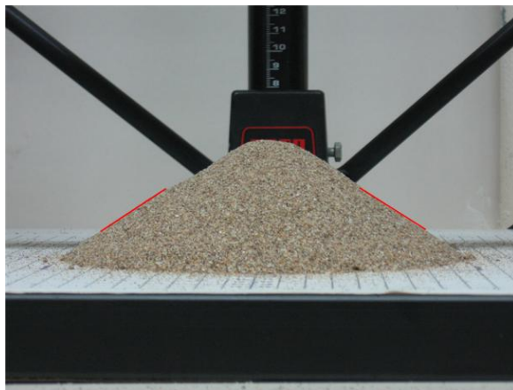
Figure 5.12. Measurement technique of the angle of repose
