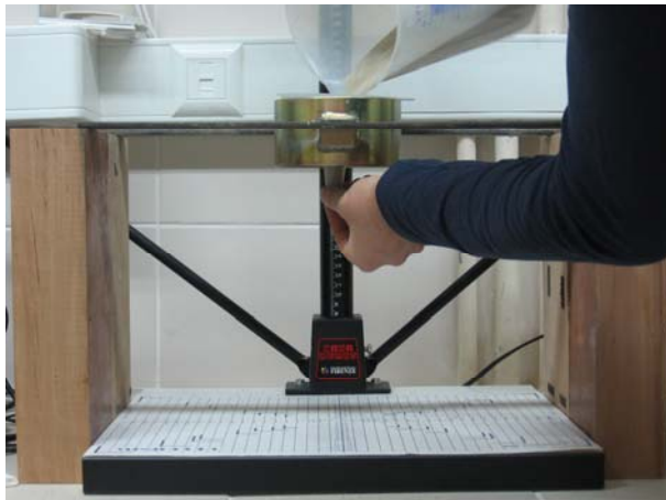
Figure 5.8. Pouring of the sand
