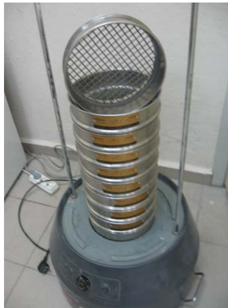
Figure 3.7. Stack of sieves and sieve shaker
