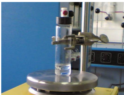
Figure 3.11. The titration set-up used for the determination of miscibility points.
