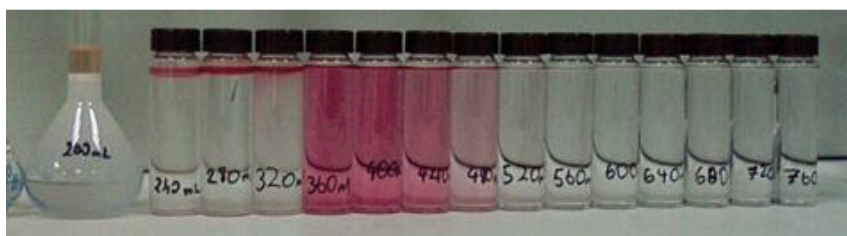
Figure 5.12. The samples collected during flushing with 60% ethanol solution at 40°C (low flow rate).
