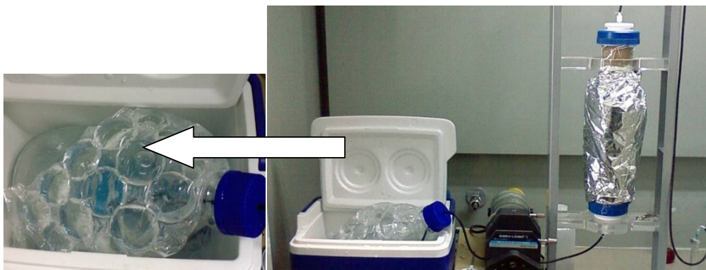
Figure 5.2. The insulated column (cooled).
