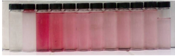
Figure 4.20. The samples collected during flushing with pure ethanol solution at high flow rate (20°C).
