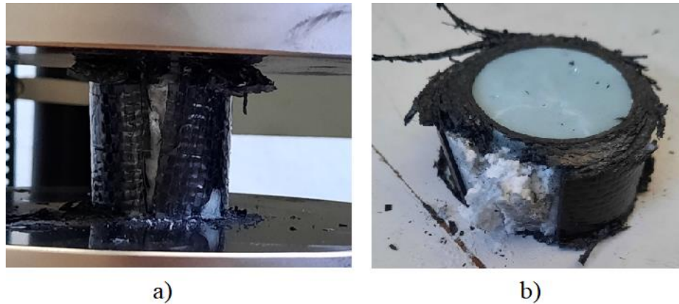
Figure 4.19. Crushing modes of Ø30mm HGMS/epoxy filled tube, a) During testing b) Final crushing mode.
