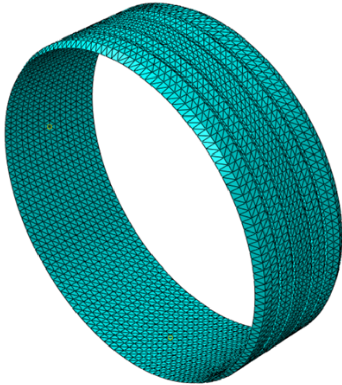
Figure 2.3. FE mesh of the tread.
