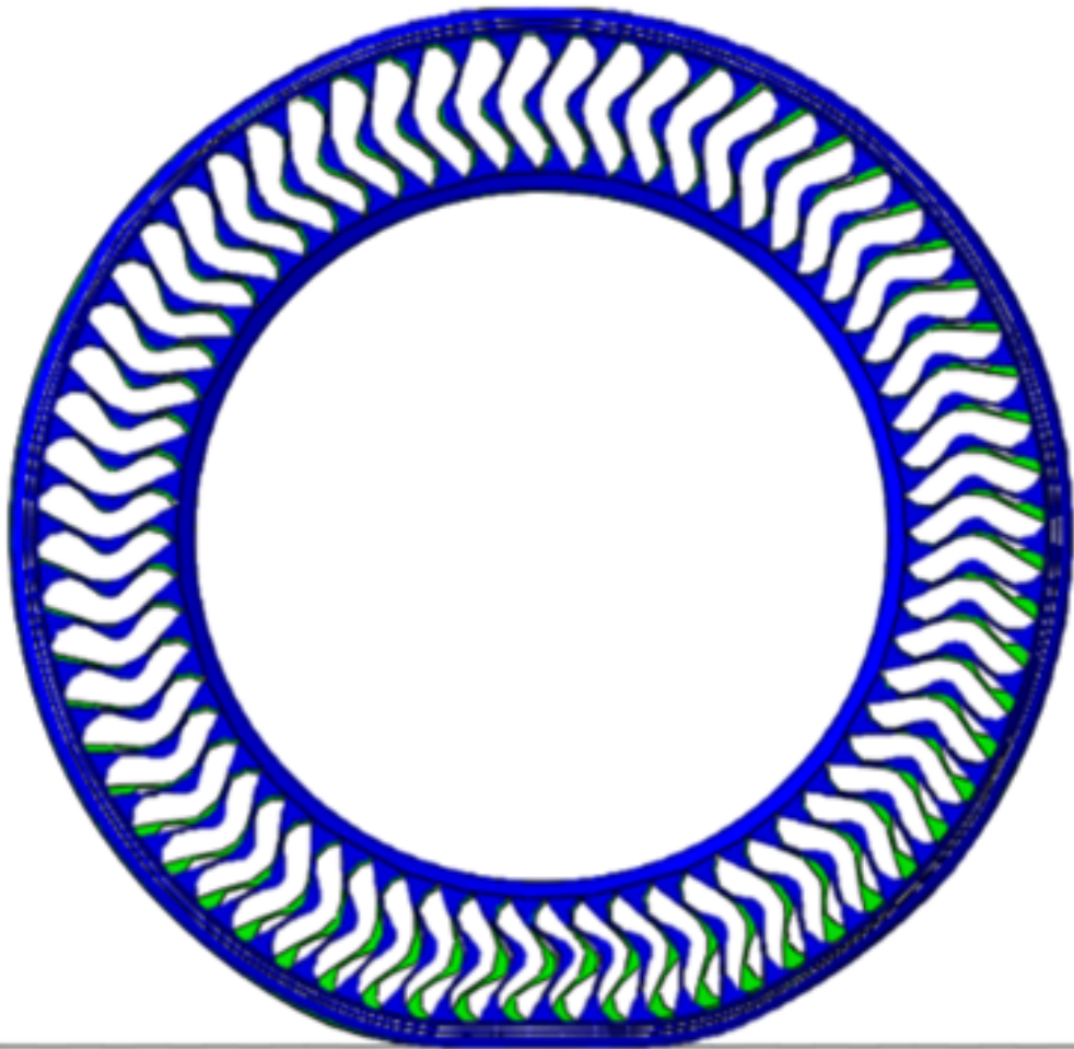
Figure 4.8. Comparison of the braking (green) and traction (blue) states of the NPT.
