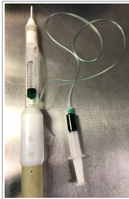
Figure 3.1 A 10 cc syringe containing 1 mL of urease solution was placed in an animal bed and 3 cc of hyperpolarized sample was injected into the magnet with a connection line from out of the magnet, in order not to move the bed during scan.
