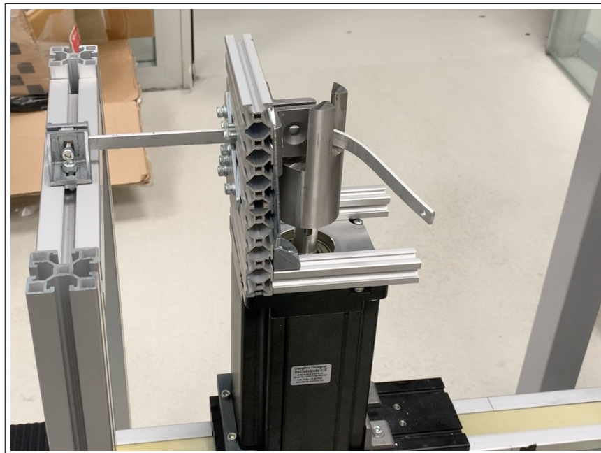
Figure 4.2 The real time bending procedure with designed system by GUI.
