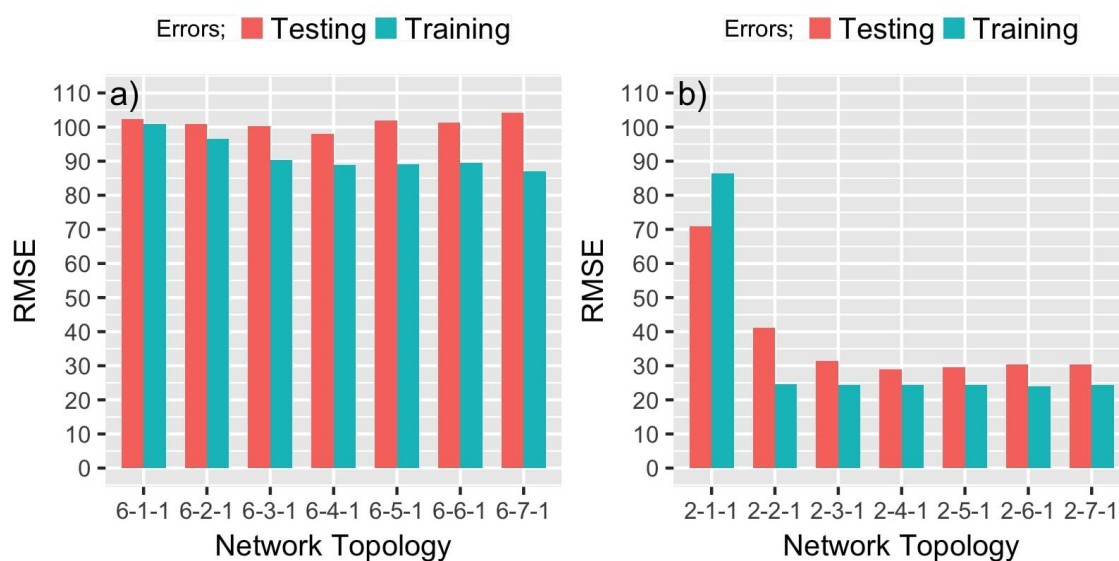
Figure 3.5. Network topologies for gravimetric CH 4 delivery a) using user defined descriptors b) using structural properties.
