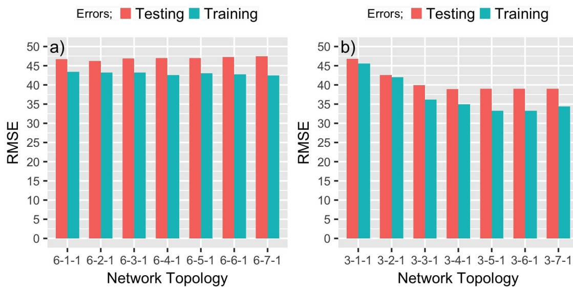
Figure 3.8. Network topologies for volumetric CH 4 uptake a) using user defined descriptors b) using structural properties.
