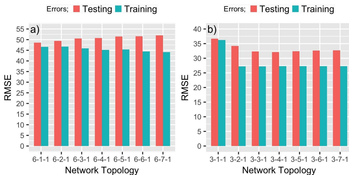
Figure 3.7. Network topologies for volumetric CH 4 delivery a) using user defined descriptors b) using structural properties.
