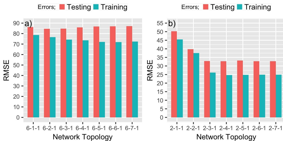
Figure 3.6. Network topologies for gravimetric CH 4 uptake a) using user defined descriptors b) using structural properties.
