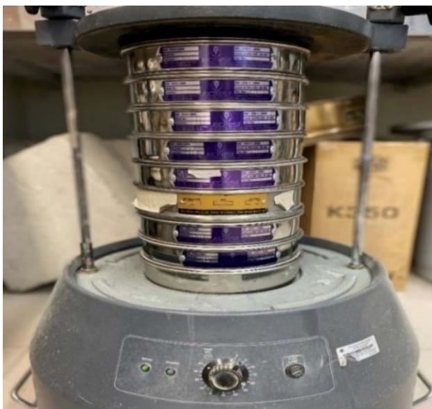
Figure 3.3. a) Endecotts EFL 2000 vibrating shaker with the mesh stack on it b) Mesh with soil sample
