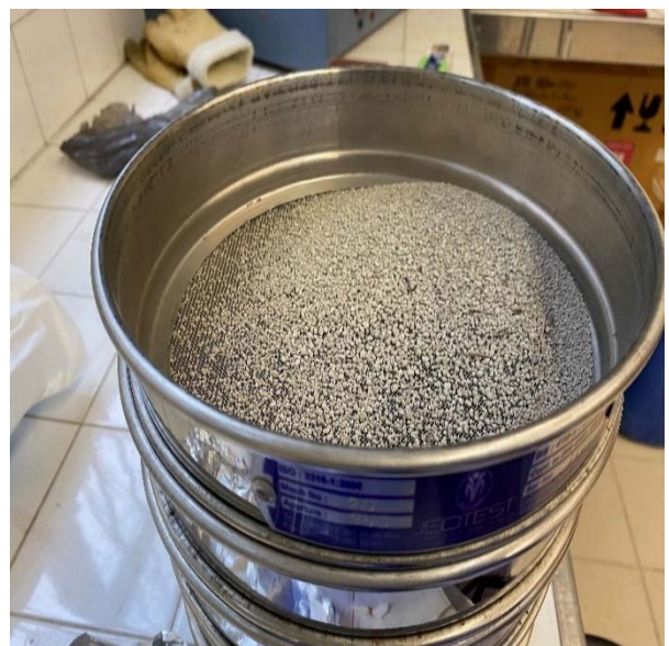
Figure 3.3. a) Endecotts EFL 2000 vibrating shaker with the mesh stack on it b) Mesh with soil sample
