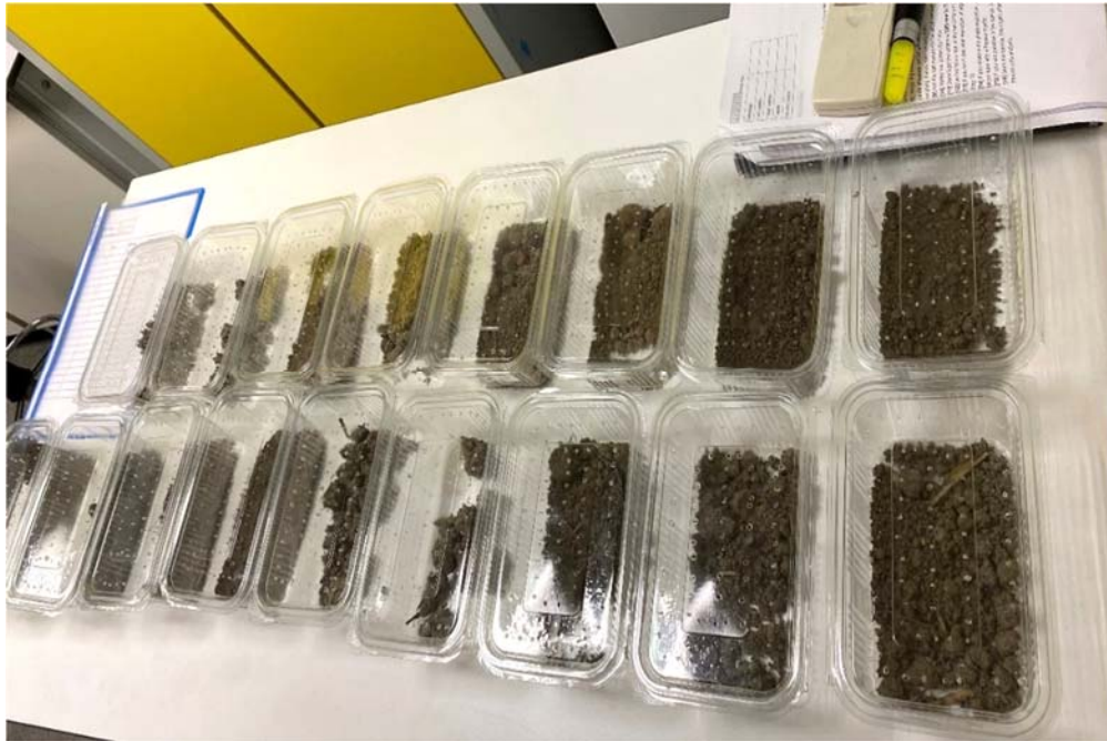
Figure 3.2. Air-drying process of soil samples in plastic containers
