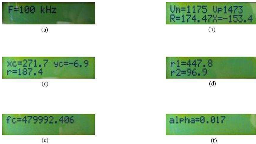
Figure 4.13 The pictures of the measured parameters displayed on the LCD. (a) Adjusted frequency (b) Real and Imaginary parts of the complex impedance (c) Center coordinates of the Cole-Cole plot (d) R_0 and R_\infty (e) Characteristic frequency (f) \alpha .
