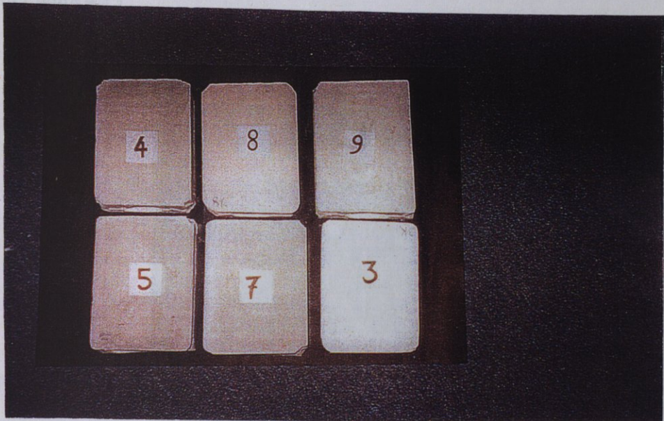
Figure 4.14. Casting molds assembled
