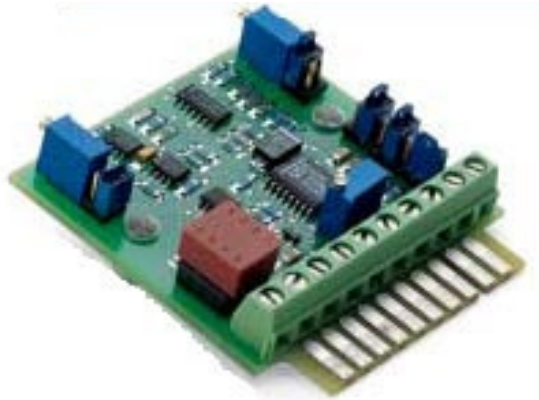
Figure 14.4. Signal conditioner module [25]
