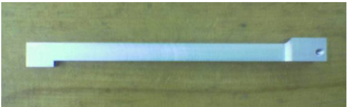
Figure 13.14. Upper arm of the extensometer
