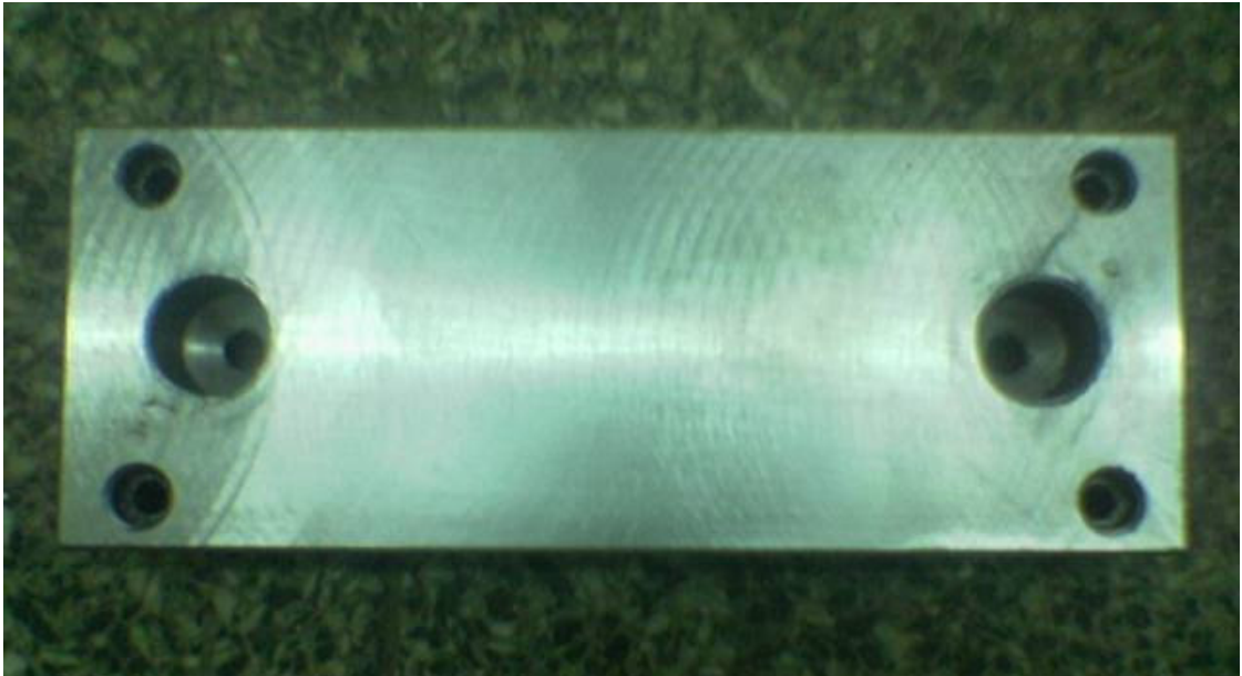
Figure 13.5. The upper base plate after machining processes
