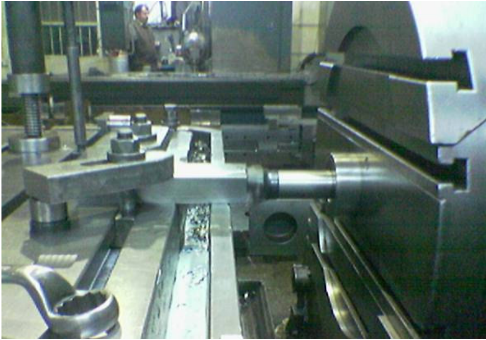
Figure 13.2. The upper base plate during milling process for its lateral faces
