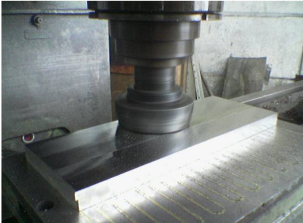
Figure 13.1. The lower base plate during milling process
