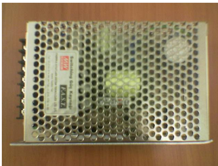
Figure 14.6. Switching power supply in the design
