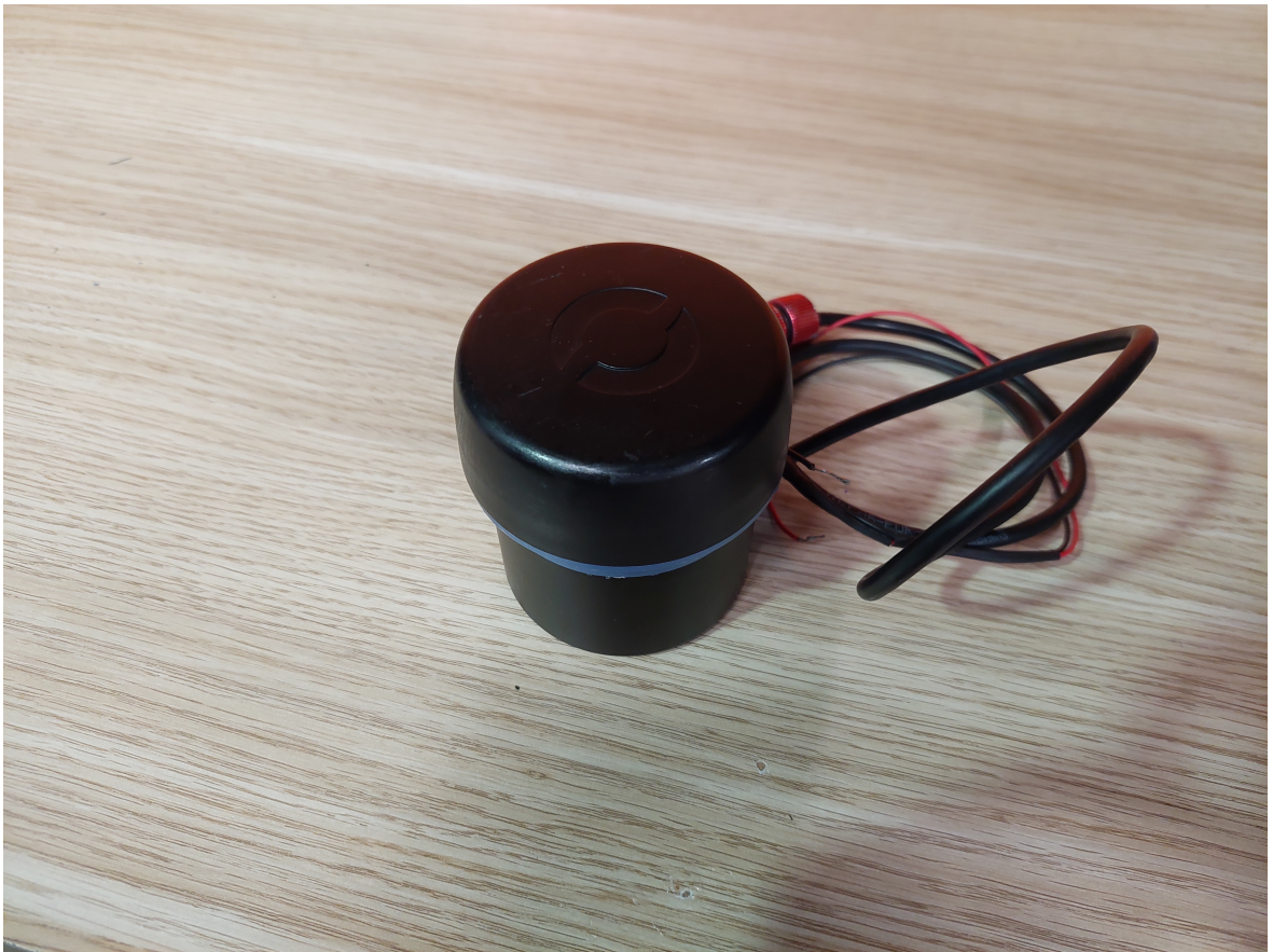
Figure 3.6. Ping-360 sonar by BlueRobotics.
