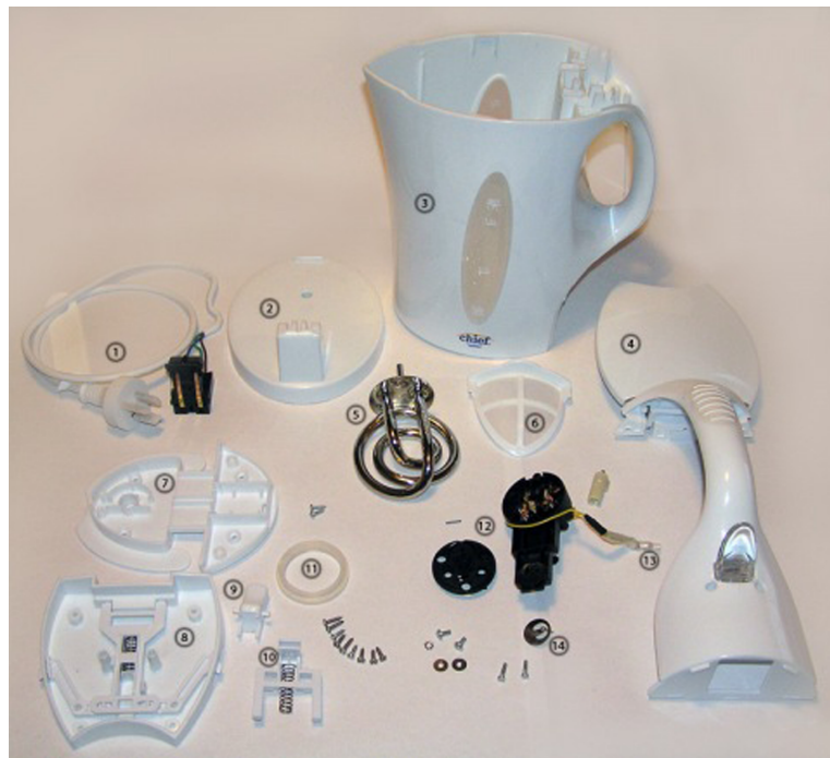
Figure 1.10. Parts of the kettle; 1. Power cable with Strix P69 Cordless System, 2. Base moulding, 3. Water reservoir, 4. Handle with lid mechanism, 5. Heating Element, 6. Removable filter, 7. Bottom of base moulding, 8. Lid release mechanism, 9. Lid release button, 10. Lid release mechanism, 11. Rubber seal, 12. Strix R72 kettle control, switch and thermal fuse, 13. LED, 14. Bi-metallic disk [57].
