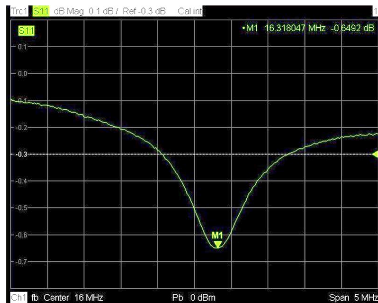
Figure 4.17. Resonance frequency caption of 6.5 turn 5 mm straight helical coil.
