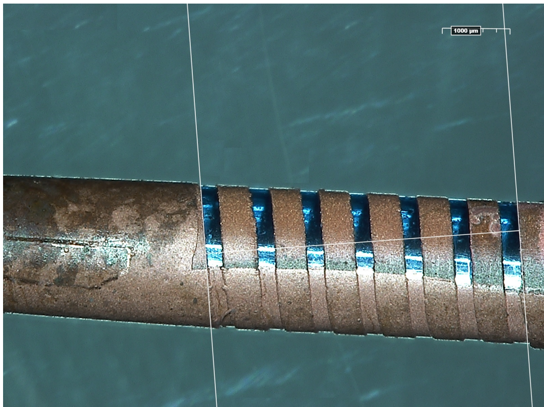
Figure 6.1. LC resonator structure fabricated on 5 Fr catheter.
