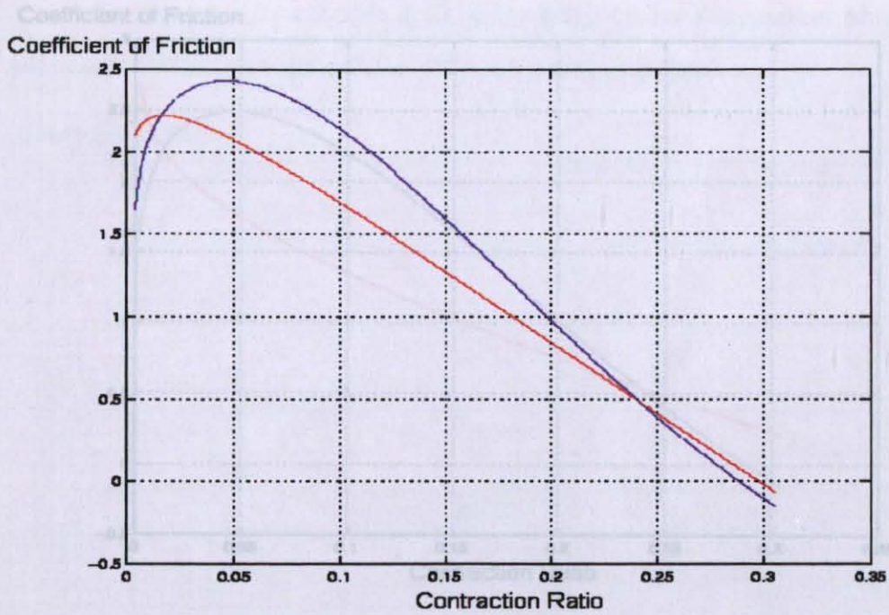
Figure 4.4 Chi-square Modeling: Coefficient of friction vs contraction ratio for 8.3 mA/sec current speed. Blue: experimental data, red: model's values.
