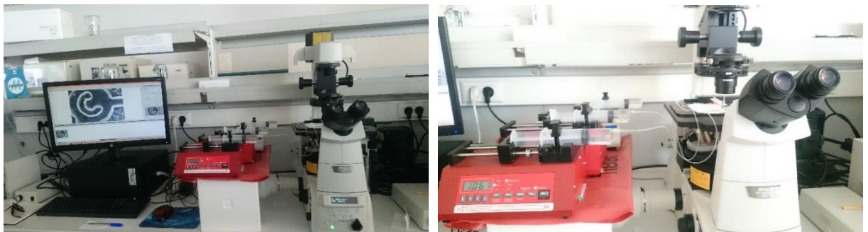
Figure 3.9. Experimental set-up system with syringe pumps and Ti inverted microscope
