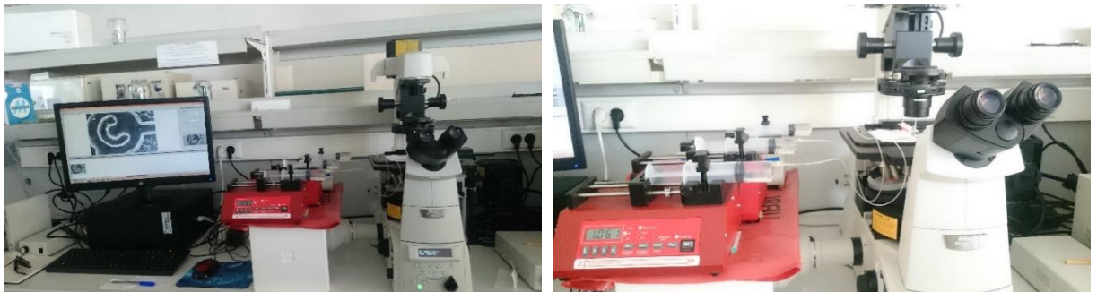
Figure 5.3. Experimental set-up system with syringe pumps and Ti inverted microscope
