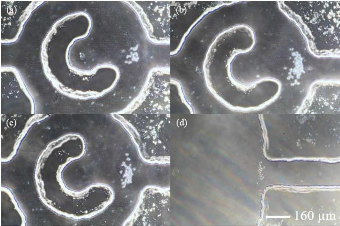
Figure 5.206. Images of (a) chamber 5 (b) chamber 6 (c) chamber 7 (d) outlet at 728th minute under magnification of 20X
