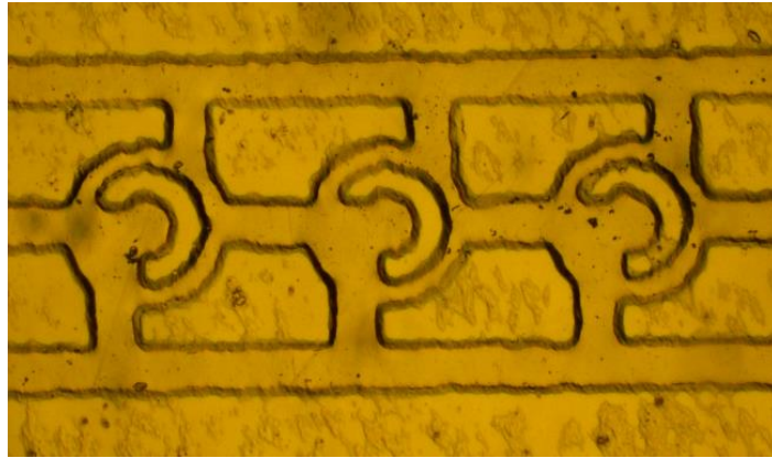
Figure 3.4. The image of the chambers on hot embossed PS piece at 10X
