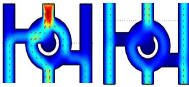
Figure 4.60. Velocity field of the first and the last chambers of model 5 for new design-2.
