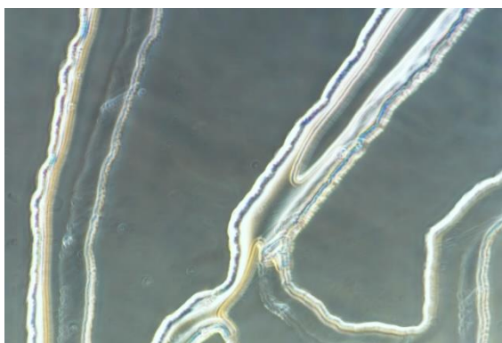
Figure 4.42. The auto white image of the backflow in the middle inlet channel of COP made device (20X objective).
