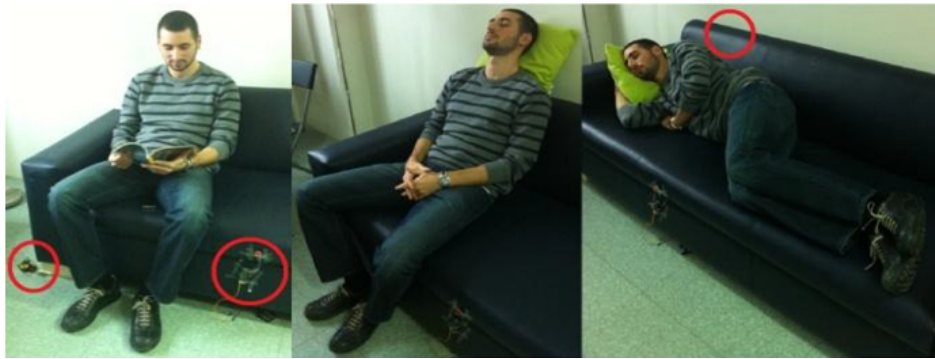
Figure 3.5. Sensor setup and a screenshot from the experiments (from left to right: FSR, accelerometer and vibration sensor).
