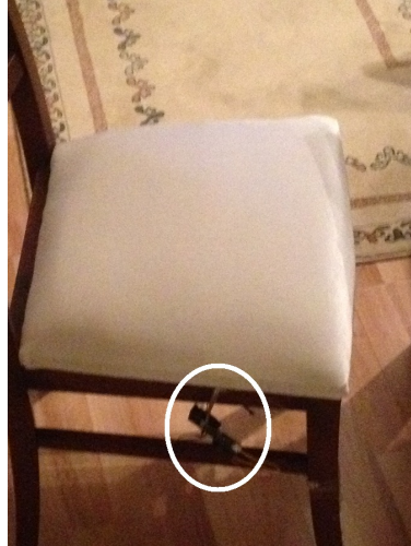
Figure 4.18. FSR located under the upholstery of chair.
