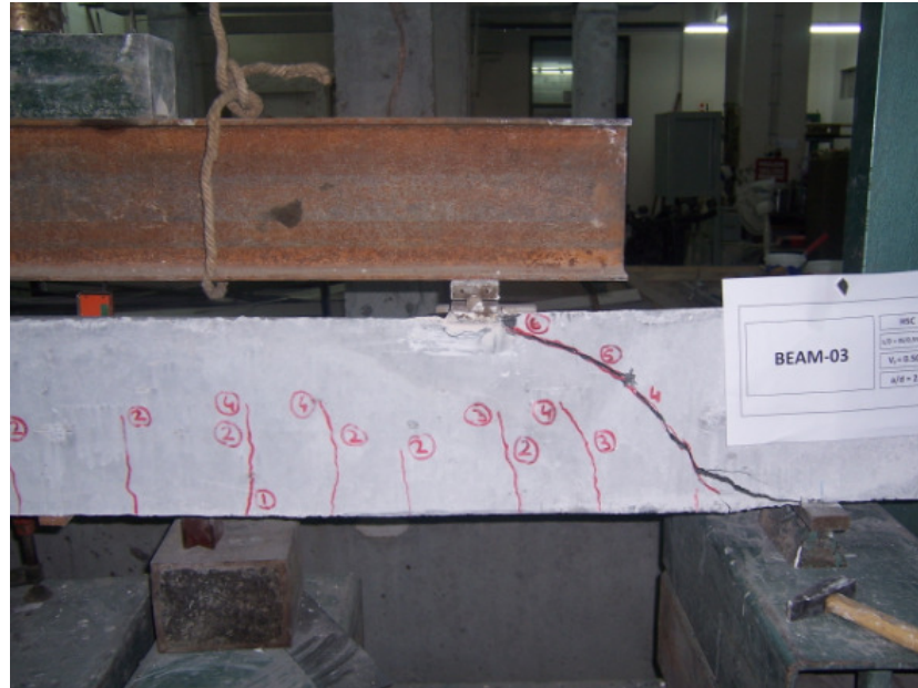
Figure 4.10. Damaged shape of the specimen BEAM-03
