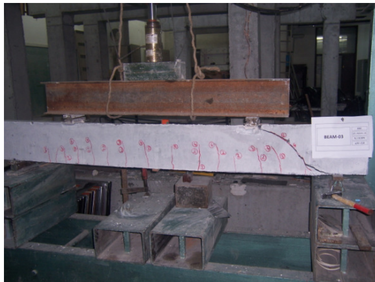
Figure 4.9. Crack propagation and damaged shape of the specimen BEAM-03
