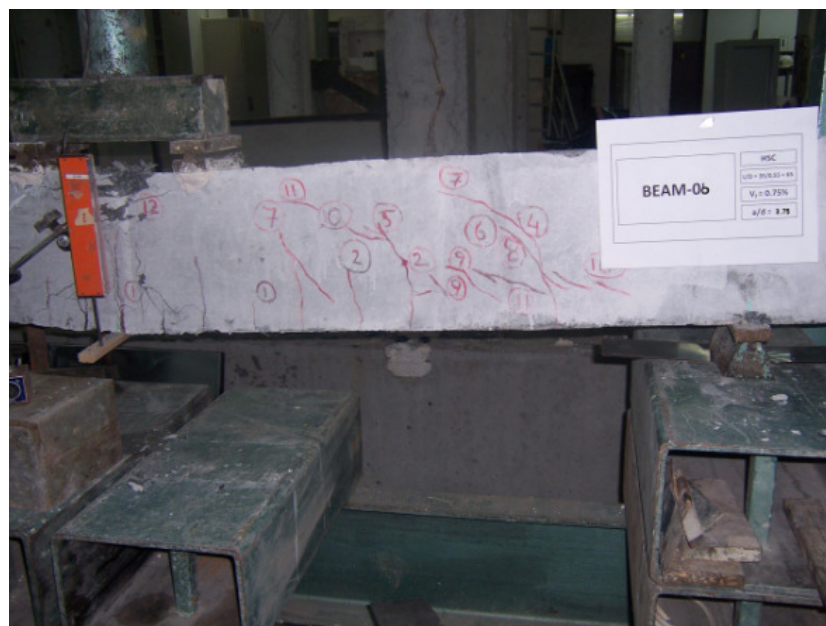
Figure 4.21. Crack propagation and damaged shape of the specimen BEAM-06
