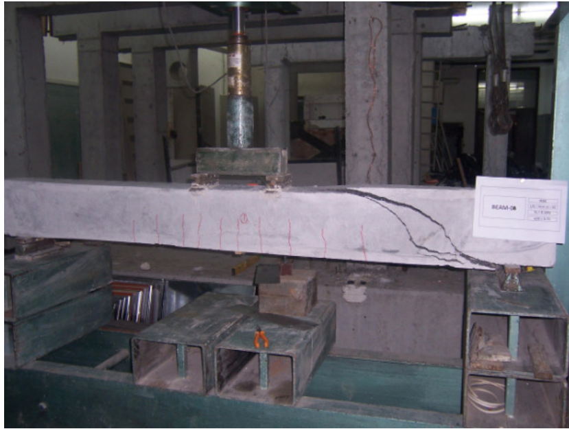
Figure 4.28. Crack propagation and damaged shape of the specimen BEAM-08
