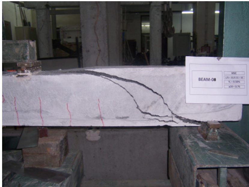
Figure 4.29. Damaged shape of the specimen BEAM-08
