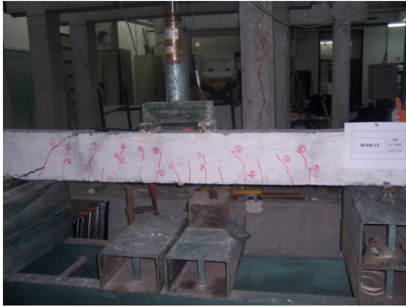
Figure 4.45. Crack propagation and damaged shape of the specimen BEAM-12
