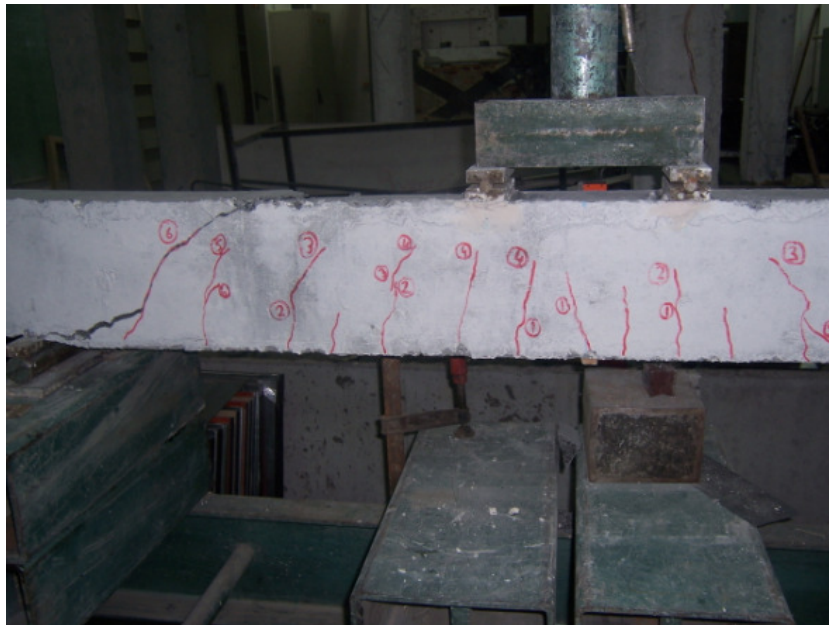
Figure 4.46. Damaged shape of the specimen BEAM-12
