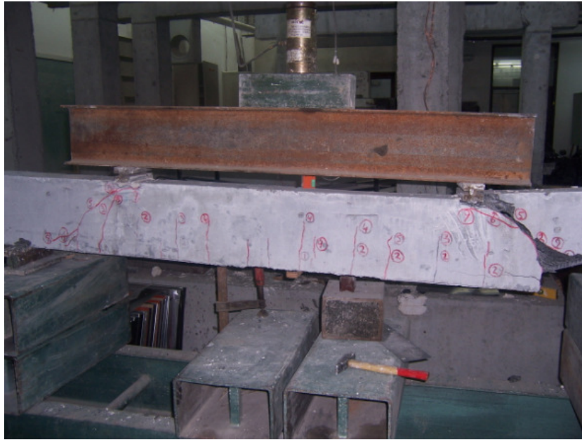
Figure 4.1. Crack propagation and damaged shape of the specimen BEAM-01
