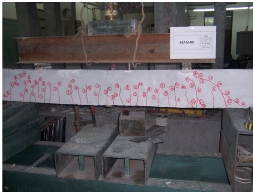
Figure 4.32. Crack propagation on the specimen BEAM-09
