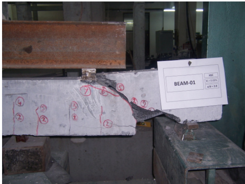
Figure 4.2. Damaged shape of the specimen BEAM-01
