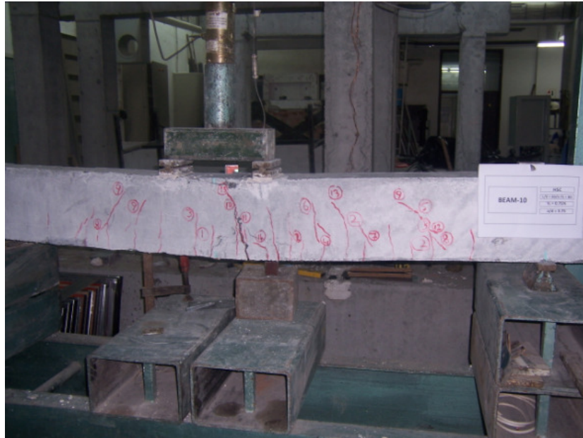
Figure 4.37. Crack propagation and damaged shape of the specimen BEAM-10
