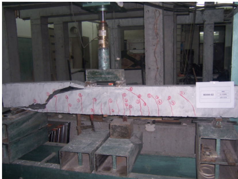
Figure 4.5. Crack propagation and damaged shape of the specimen BEAM-02
