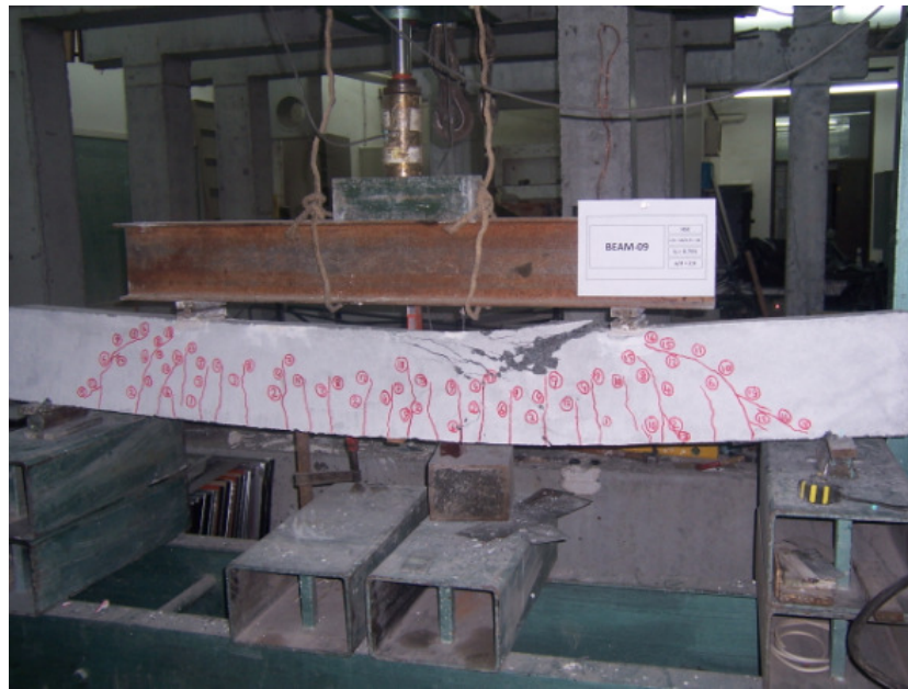
Figure 4.33. Crack propagation and damaged shape of the specimen BEAM-09
