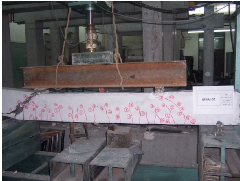
Figure 4.24. Crack propagation and damaged shape of the specimen BEAM-07
