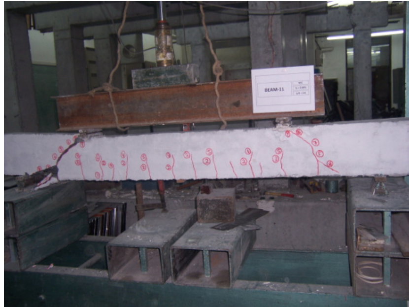
Figure 4.41. Crack propagation and damaged shape of the specimen BEAM-11
