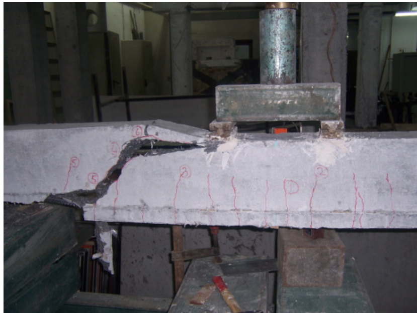
Figure 4.14. Damaged shape of the specimen BEAM-04
