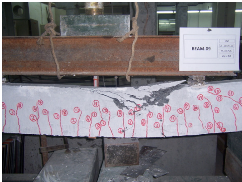
Figure 4.34. Damaged shape of the specimen BEAM-09
