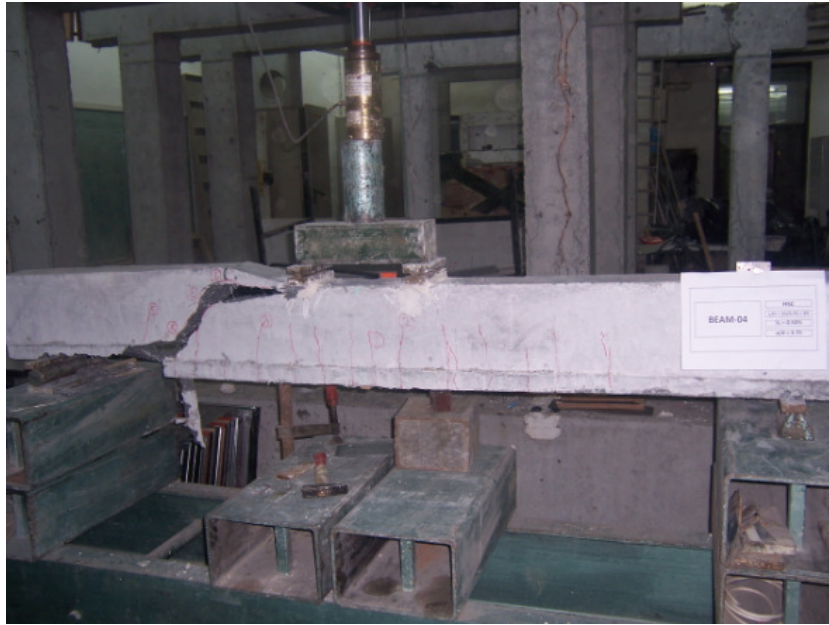
Figure 4.13. Crack propagation and damaged shape of the specimen BEAM-04
