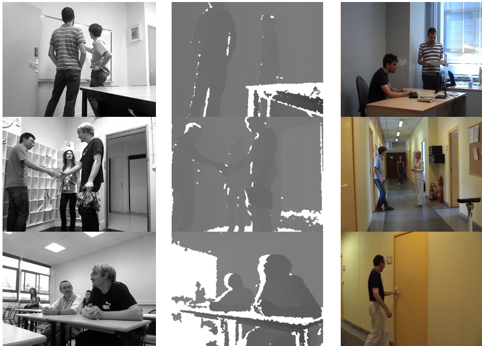
Figure 2.3. LIRIS Human Activities Dataset [3] is one pioneering multi-modal dataset in that it contains complex human activities in a realistic setting. From left to right, gray scale images captured by Kinect, their corresponding depth images and color images from the Sony camcorder are illustrated respectively.
