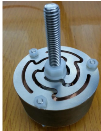
Figure 3.16. Measured Resonator with Small Ring Magnet Inside.
