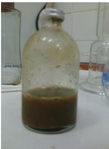
Figure 4.1. 120 ml serum bottle with 40 ml active volume.
