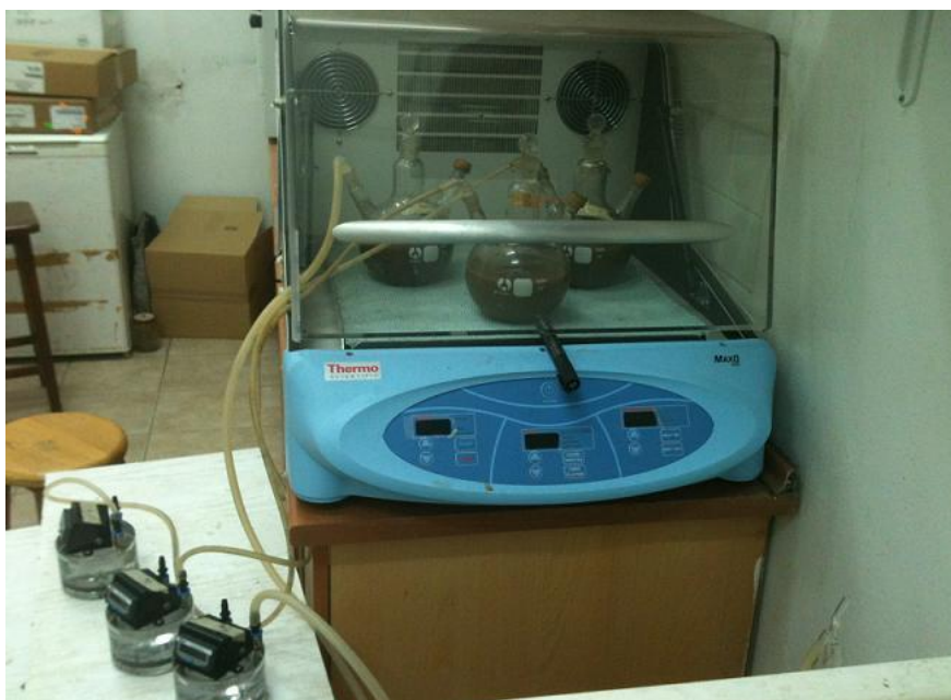
Figure 4.2. Digesters placed on the temperature controlled incubator shaker.
