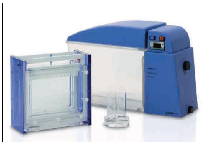
Figure 4.5. DGGE equipment used in the study (Ingeny phorU)
