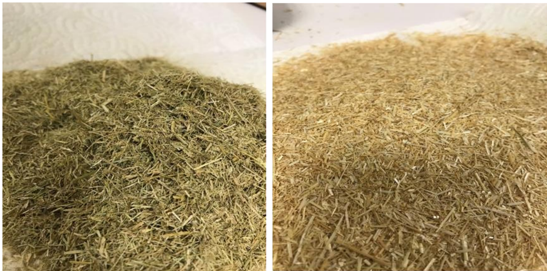
Figure 4.1. The substrates after being ground to 5-10-mm particles; rice straw and wheat straw.
