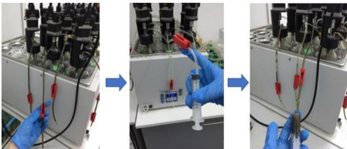
Figure 4.7. Samples collected from digesters on days 0, 3, 5, and 30 to observe the VFA production and the depletion in the acidogenesis phase.
