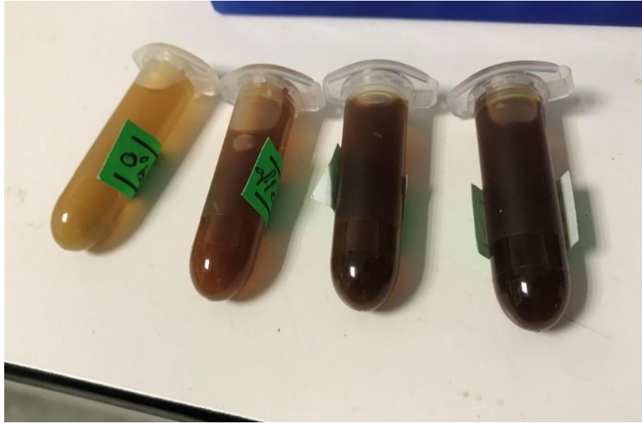
Figure 5.3. Filtrates released after 24 h pre-treatment of rice straw by 0 %, 4 %, 6 %, and 8 % NaOH dosages, respectively.
