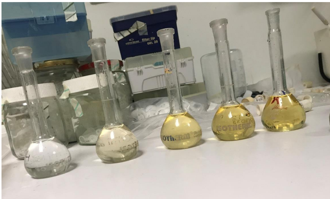
Figure 5.4. Differences in color of diluted filtrates of pre-treated rye straw samples with 0 %, 4 %, 6 %, 8 %, and 10 % NaOH dosages, respectively.
