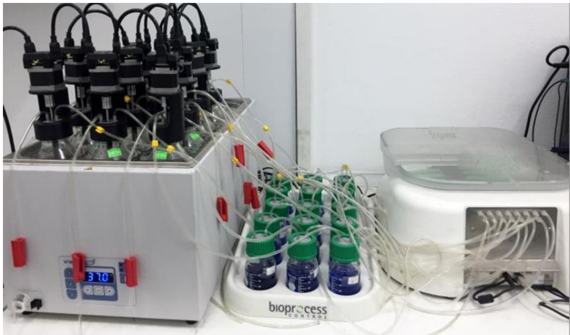
Figure 4.6. Automated Methane Potential Test System II (AMPTS II).
