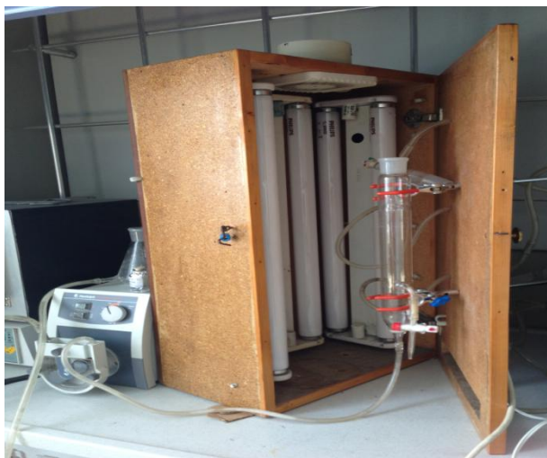
Figure 3.8. Irradiation box for the experiments under visible light irradiation.
