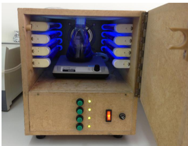
Figure 3.5. Irradiation box for the experiments under UV irradiation.
