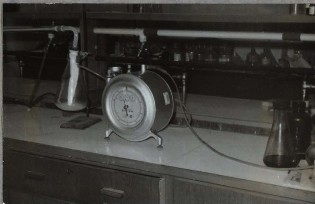
Figure 8: The Connection of the Gas Meter to the Filter Bag
