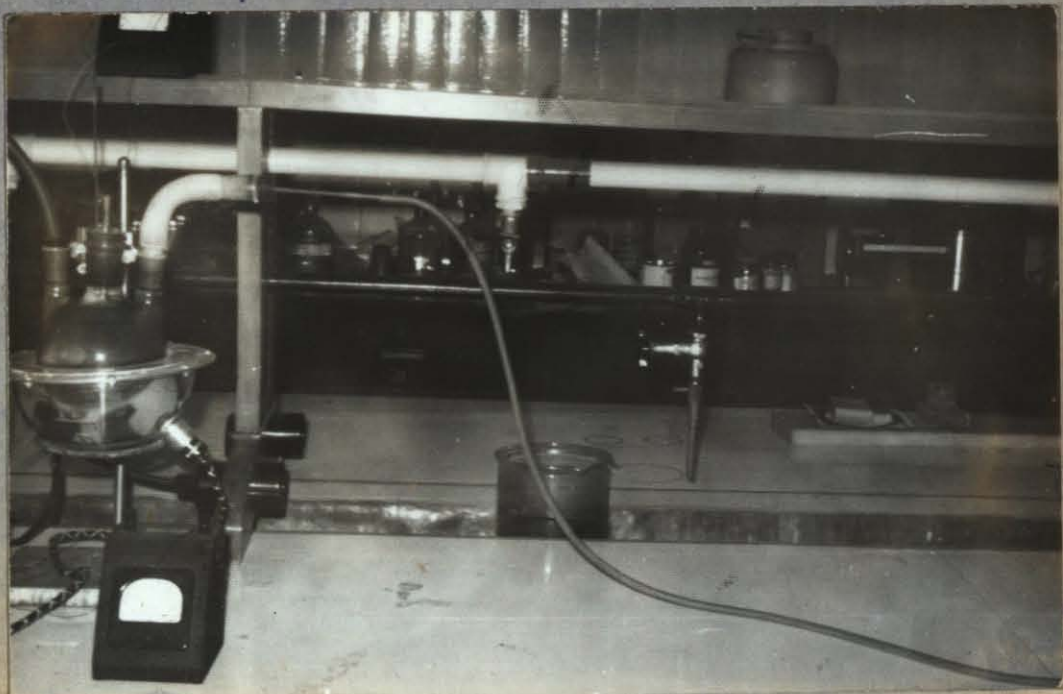
Figure 5: Collecting Part (below 320^{\circ}\text{C} )
