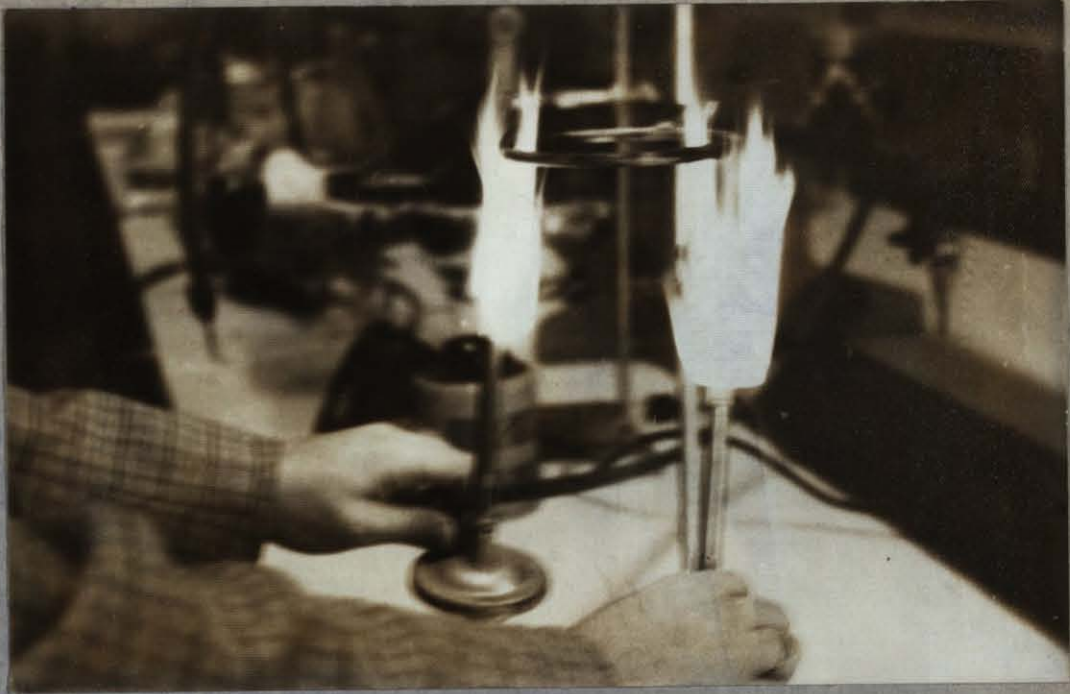
Figure 11: The Two Pieces of PVC, When Exposed to Flame
