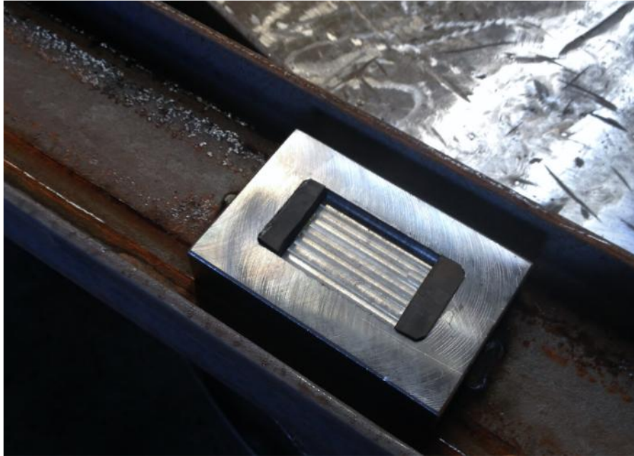
Figure 2.32. View of roller bearing shelter with rubber strip stoppers on both side (Sekman, 2016).
