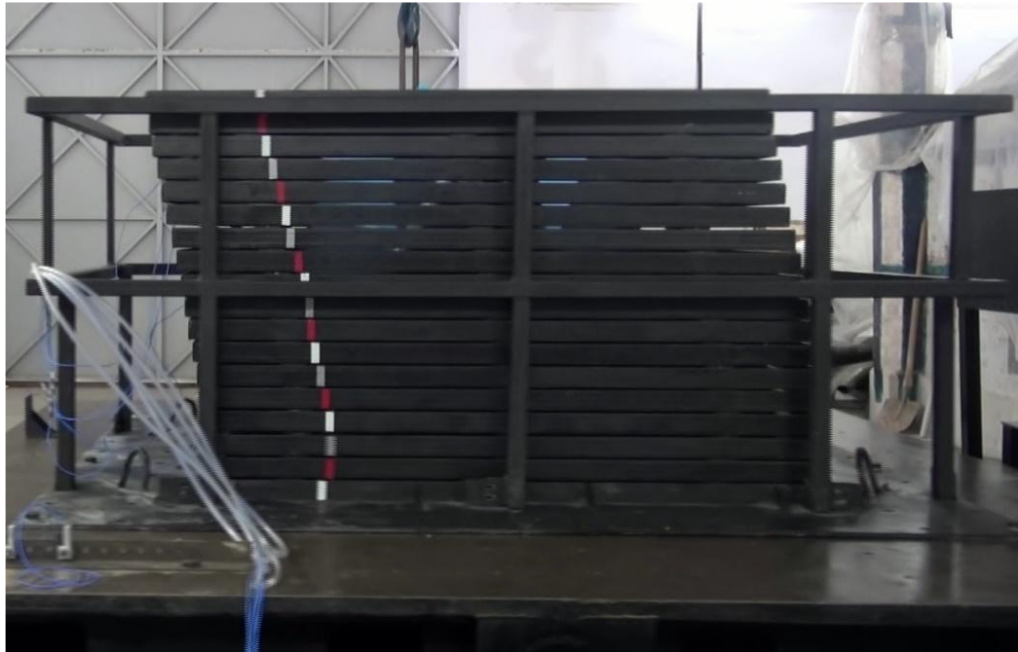
Figure 2.31. Side view of unidirectional laminar box utilized in this study (Sekman, 2016; Goztepe, 2016).
