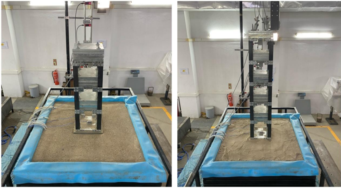
Figure 3.12. Building models of 1:10 Scaled 3-Story (left) and 5-Story (right) structures.
