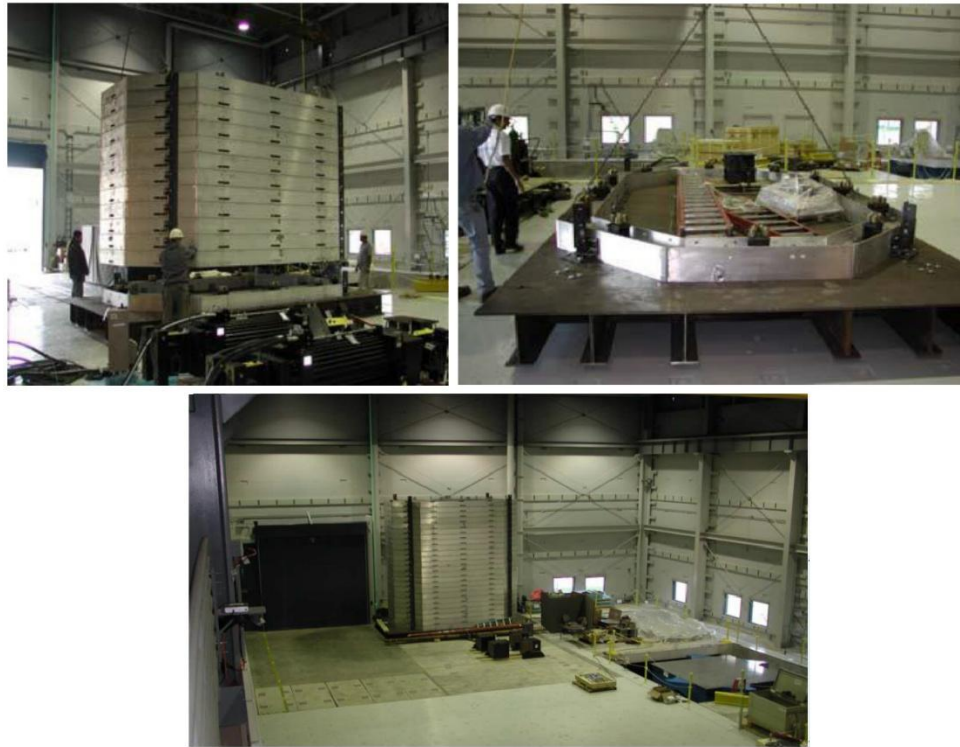
Figure 2.30. A large-scaled laminar shear box, base plate, and during shaking table experiment (Thevanayagam and Ecmis, 2006).
