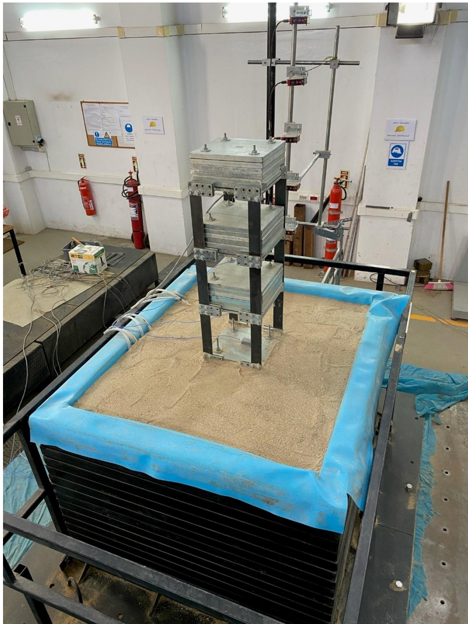
Figure 3.23. An example of the 3-story test setup before performing an earthquake scenario.
