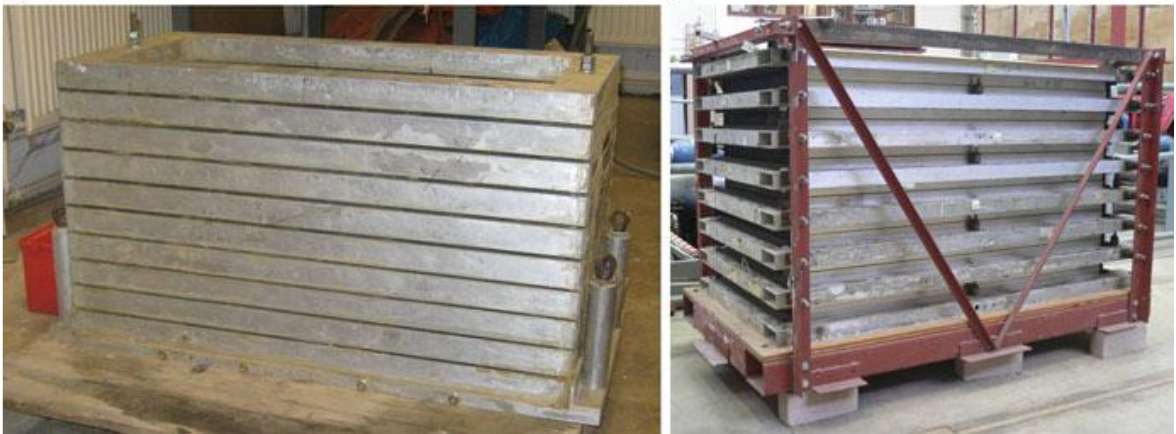
Figure 2.23. Examples of equivalent shear beam container: ESB used in centrifuge testing, University of Cambridge – left; Shear stack used in 1-g testing, University of Bristol – right (Bhattacharya et al. , 2012).
