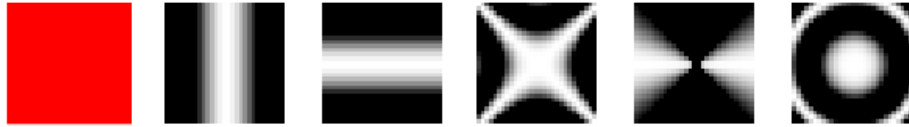
Figure 2.1. Visual filters. Left to right: Color, vertical, horizontal, hyperboloid, polar, cocentric filters. The first three are considered for the case of visual filters with N_l = 3 . All are considered for the case of N_l = 6 .
