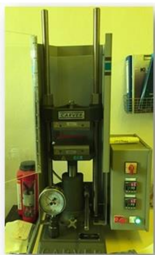
Figure 3.4. Hydraulic press machine (Carver).
