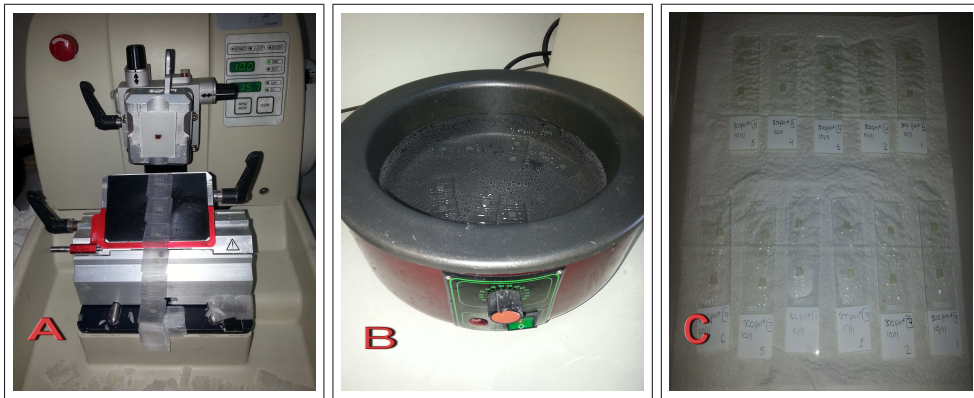
Figure 3.8 Microtoming and Slide Preparation:A: Microtome, B: Water bath, C: Tissues Aligned on Glass Slides.
