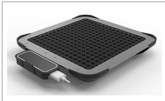
Figure 2.1 Ultrahaptics STRATOS Explore device that has 16x16 array of transducers that are transmitting 40 kHz ultrasound waves and the Leap Motion Controller device (left side) [12].
