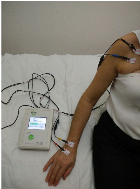
Figure 9.17 In Impedimed SFB7 clinical studies, the tetra-polar electrode measurement model is used. Two electrodes are placed on the 3 rd metacarpal bone of the DA, and two electrodes are placed at the infraclavicular fossa, 1 cm apart. The outer electrodes are used for applying current, and the inner electrodes are for sensing the voltage.
