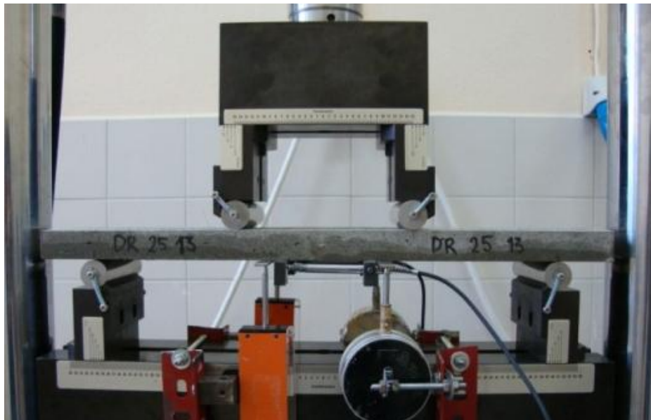
Figure 4.2. Four-point bending test setup
