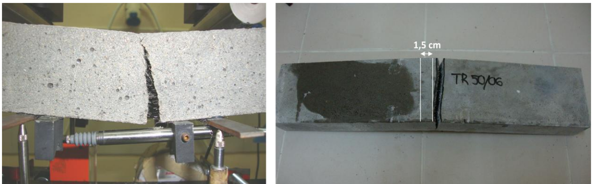
Figure 5.1. Crack region, where specimens cut for image analysis
