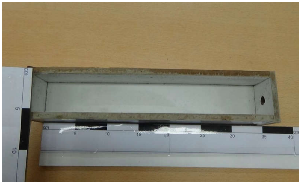
Figure 3.10. Wooden mold for casting of monolithic model piles.
