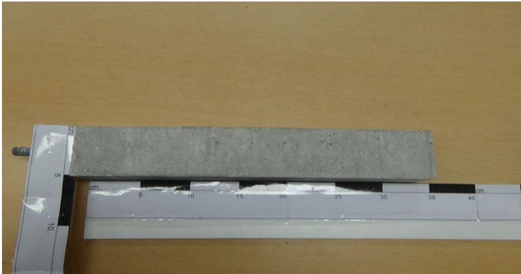
Figure 3.11. Demolded Monolithic pile.
