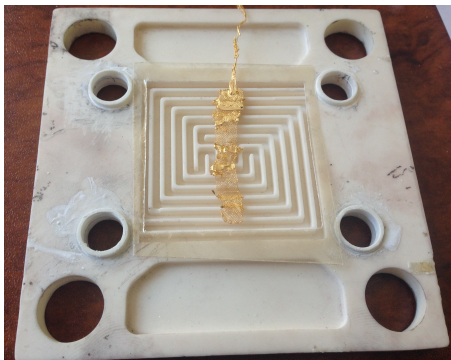
Figure 2.2. Gold mesh at the bottom of cathode layer.
