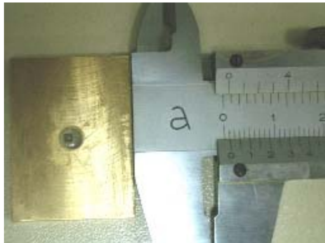
Figure 4.5 Vernier Caliper penetration method for soft RC determination
