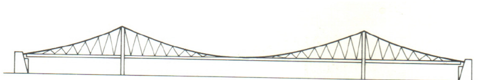
Figure 3.2. Suspension system with inclined hangers (Gimsing, 1998)
