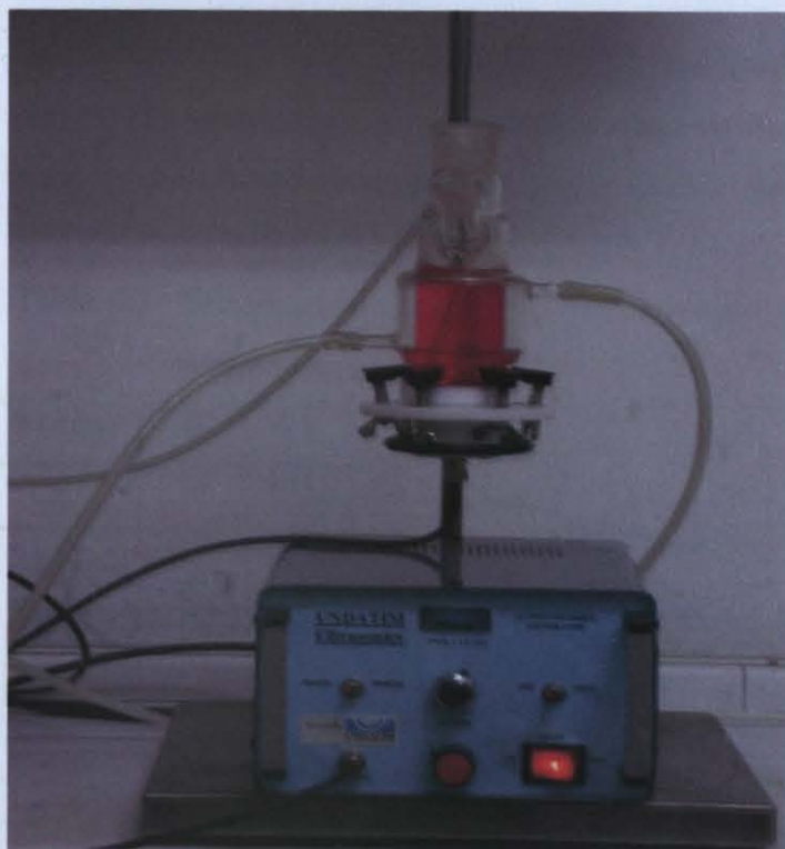
Figure 4.1. Photographic view of SYSTEM I: 300 kHz-150 mL reactor.
