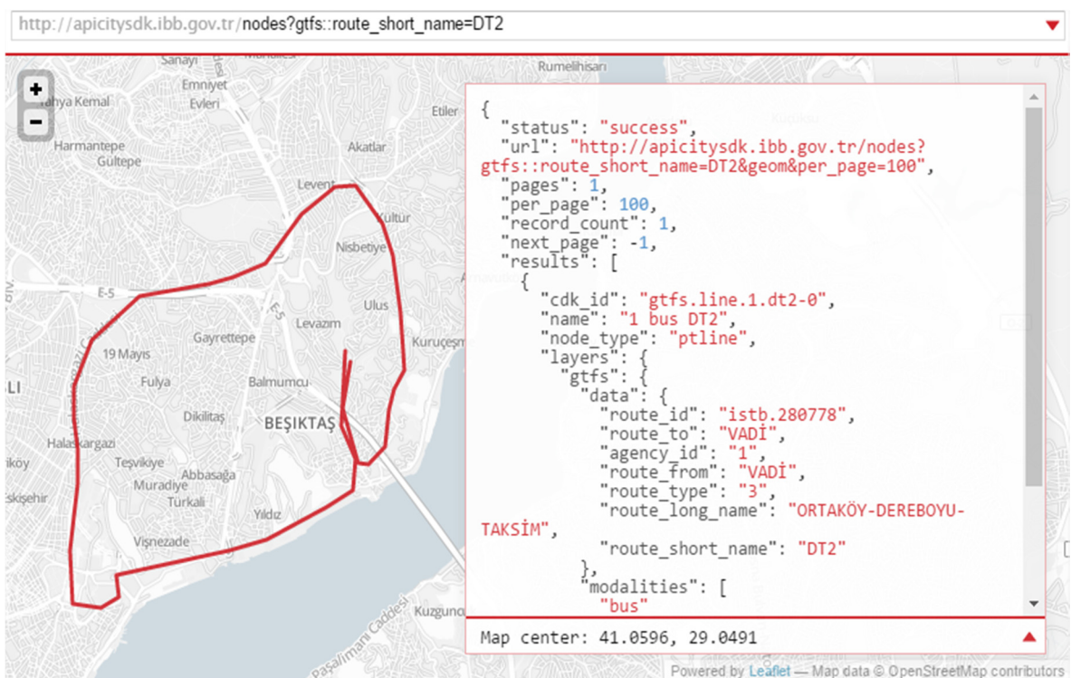
Figure 3.9. A query asking public transportation lines has a short name “DT2” in CitySDK API.
