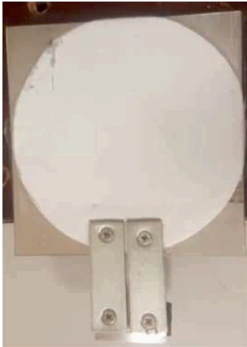
Figure 3.11. Al coated PTFE film which is fixed and it's electrical contact is established.
