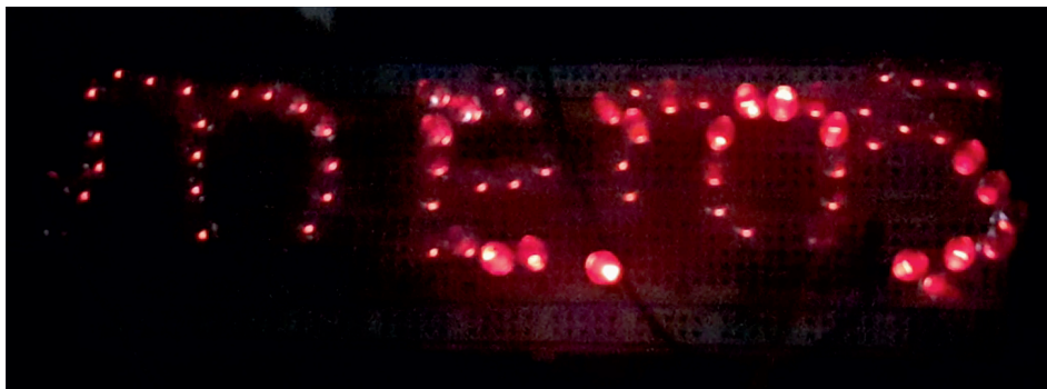
Figure 4.17. Driving LEDs with macro scale triboelectric generator.
