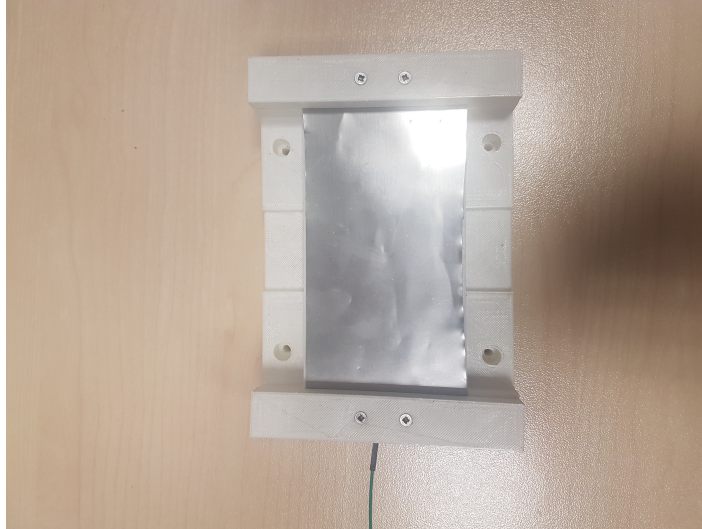
Figure 3.14. Top part of the macro scale triboelectric generator.
