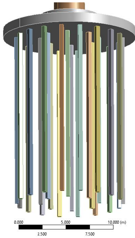
Figure 3.5. Pile Group in the Model.
