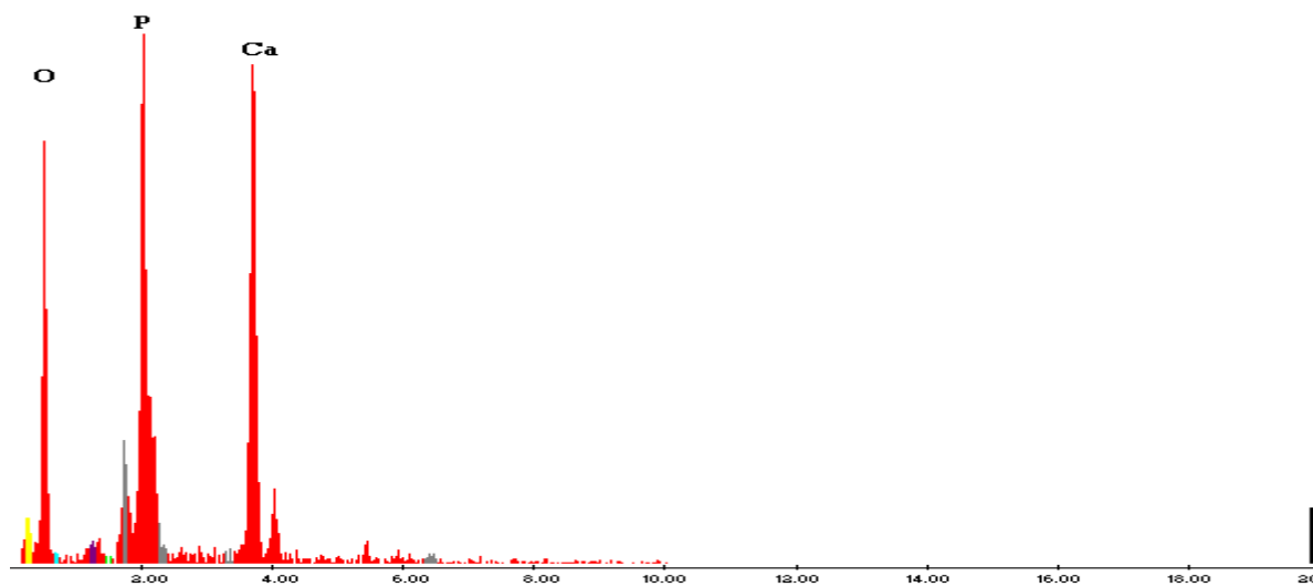
Figure 4.24. EDAX results of the sample in set 18
