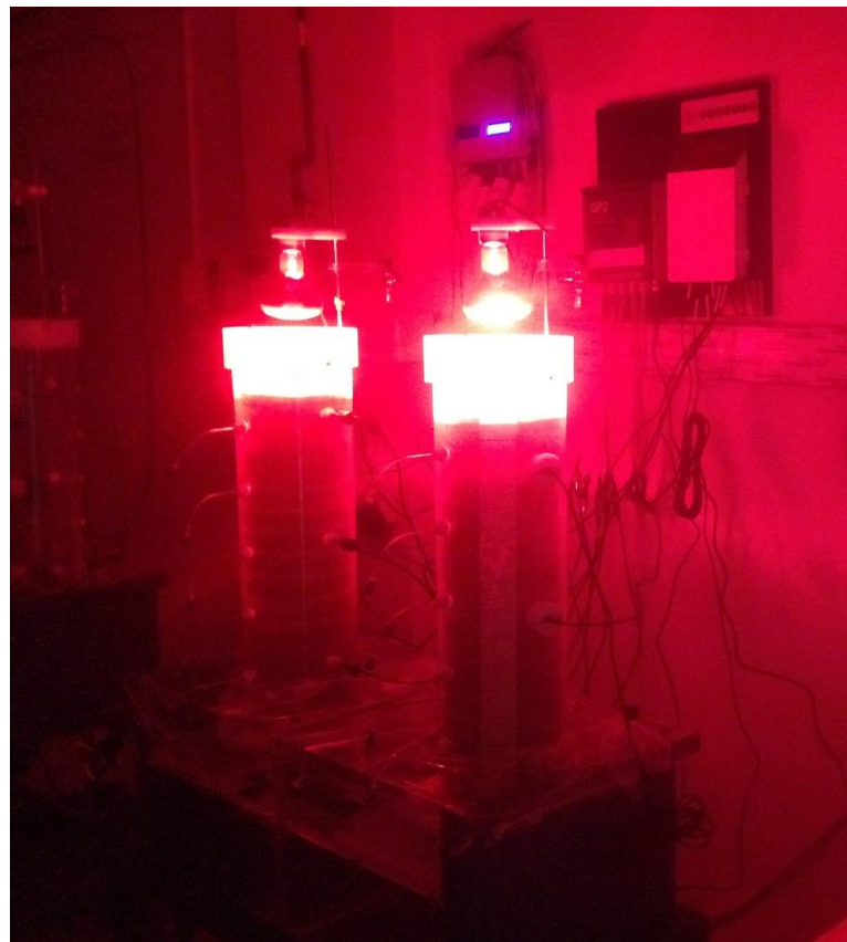
Figure 4.5. Soil columns in dark having infrared lamps controlling the soil surface temperature.
