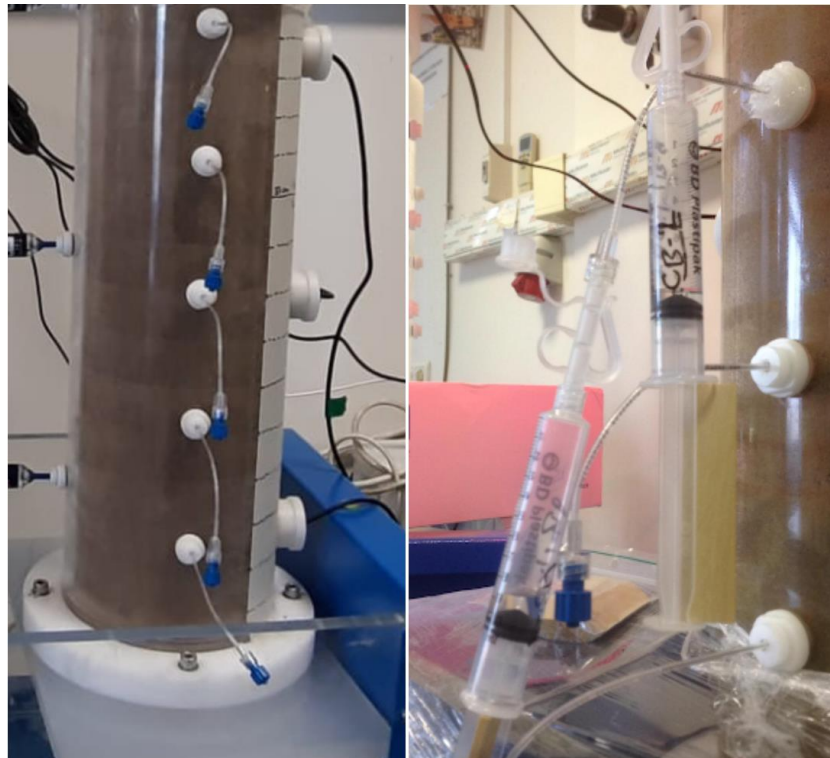
Figure 4.7. Soil water collection using the suction cups.
