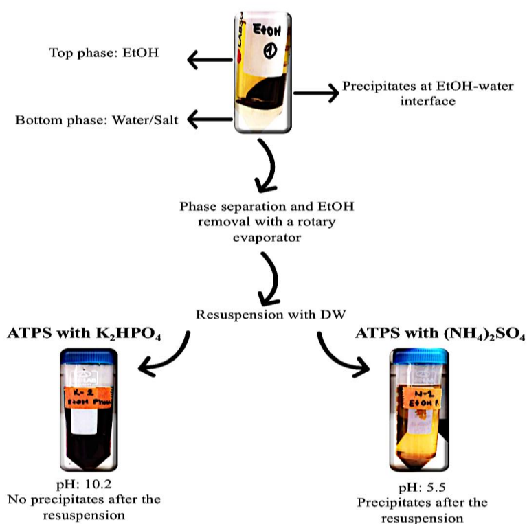
Figure 4.7. The formation of precipitates during the ATPE containing different salts.
